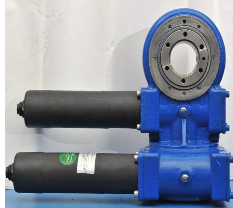
Fig 2.4: Slowing drive for active multi-axis sunlight trackers
