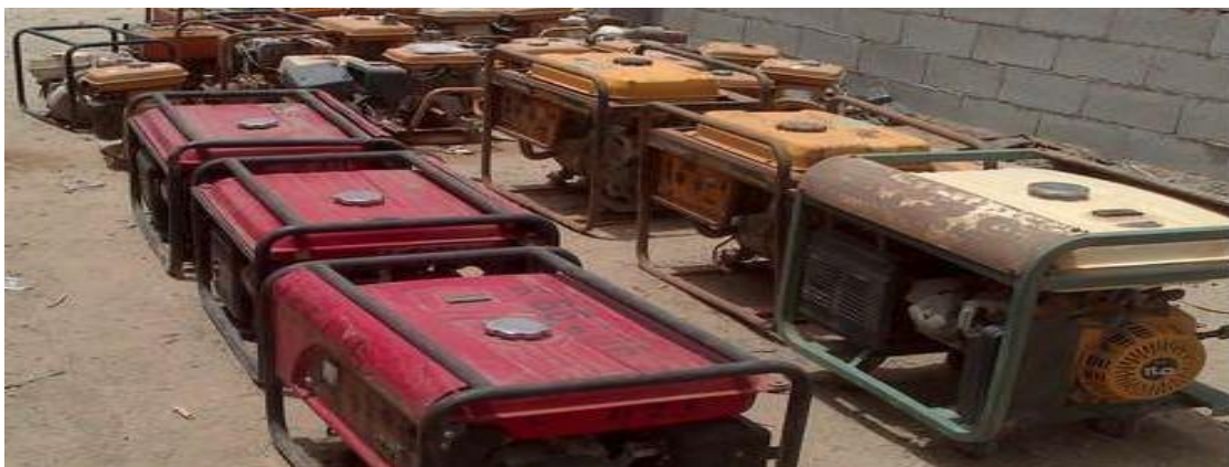
Fig 6.6: Home petrol electricity generators 1.8 kW used in Al Rakabah ( https://www.google.com/imghp )
