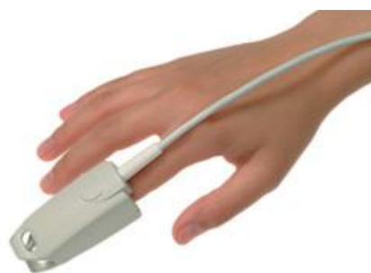
Figure 1.4: A typical reflective PPG sensor for measuring blood oxygen saturation ( SpO_2 ) and heart rate [3]
