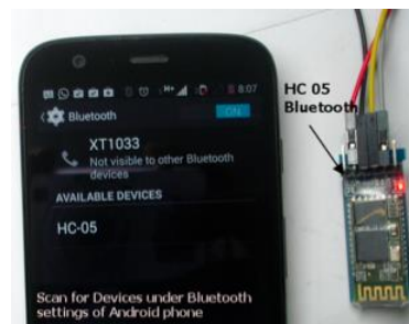
Figure 6.14: A view of the Bluetooth module while pairing it with a smartphone
