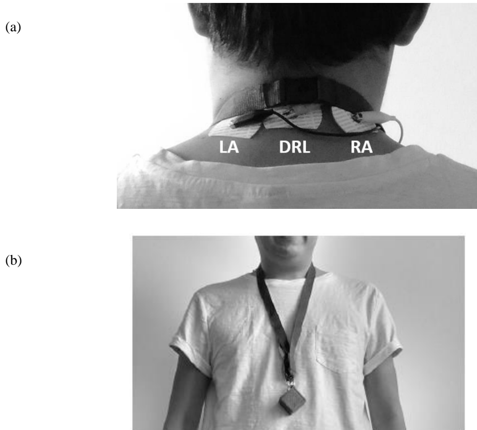
Figure 2.19: (a) The backside of the neck proposed electrode placements; (b) The subject wearing the necklace-form-1-lead ECG device [42]
