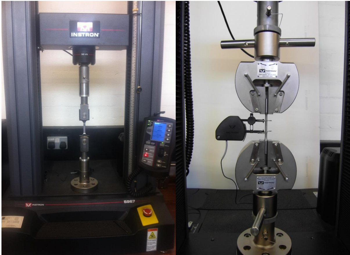
Figure 4.1: The tensile test performed on the sample.
