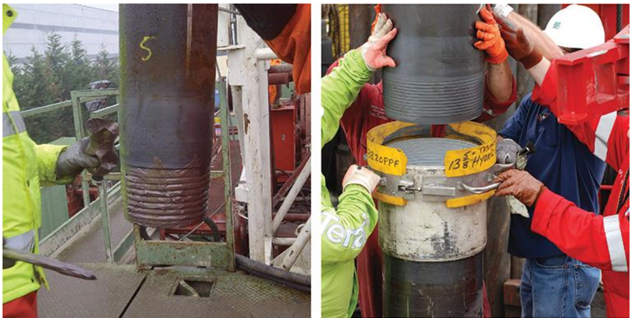
Figure 1.3: Drill pipe threaded connection. (Khiggins, 2012)
