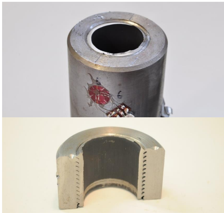
Figure 24: Failure on the threaded connection pin and box.
