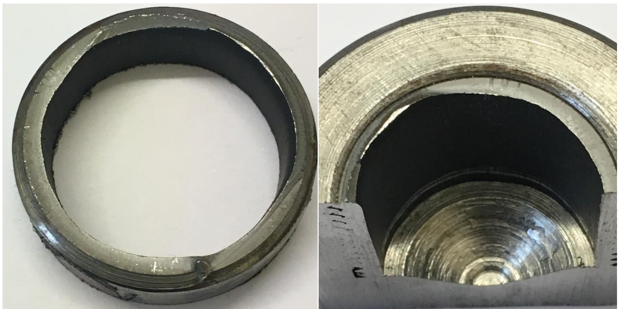
Figure 5.34: a) Fracture surface test low to high; b) zone divided by the beach marks.
