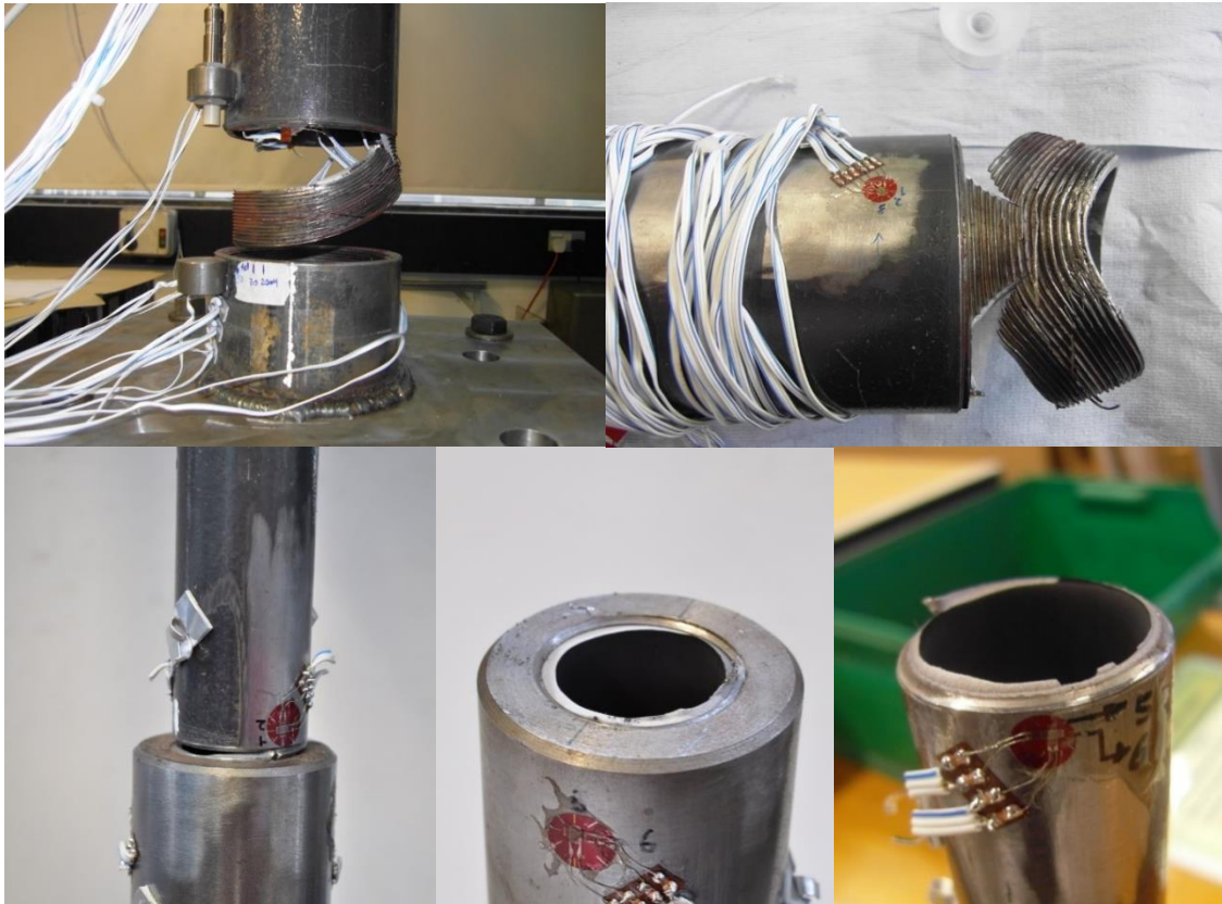
Figure 5.9: Failed 4.5" and 1" API Line Pipe specimen.
