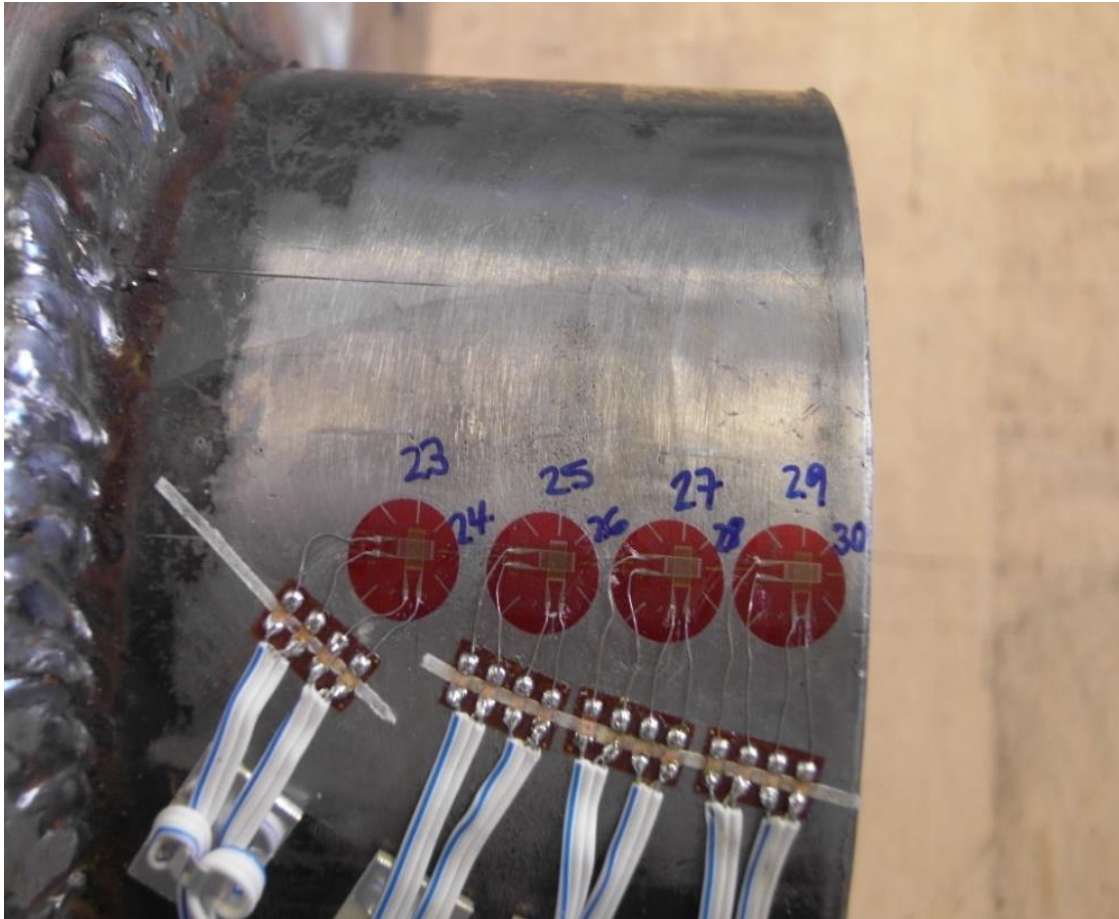
Figure 4.11: Strain gauge location on the box.
