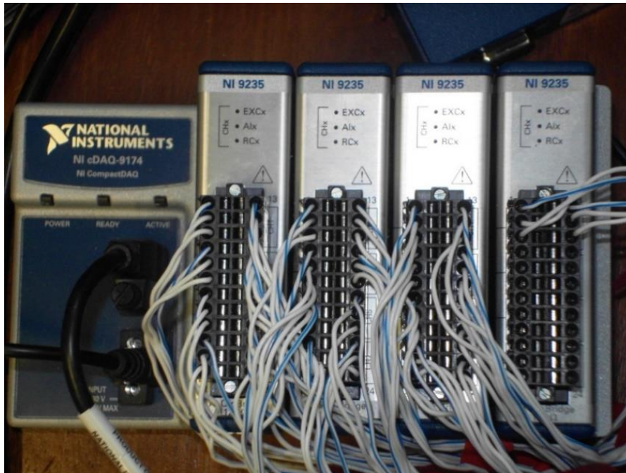
Figure 4.15: 34 strain gauge is connected to the chassis and module.
