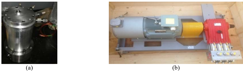
Fig. 2. Photographs of the system components. (a) CO 2 Turbine; (b) CO 2 liquid pump.
