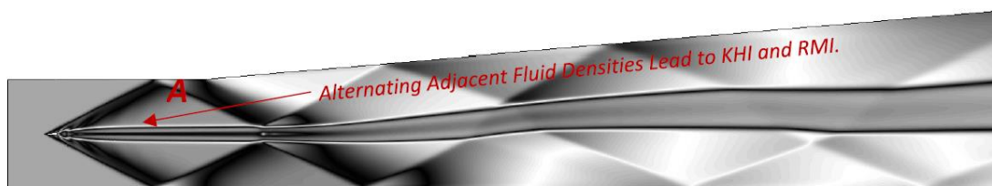
Figure 24. Shock train visualization for a single strut combustor in terms of density ( \text{kg}/\text{m}^3 ).
