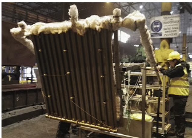
Fig. 5. Industrial set up and Thermocouple positions.
