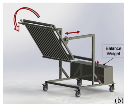
Fig. 2. The mechanical design of the FHP: (a) FHP design, (b) FHP stand.
