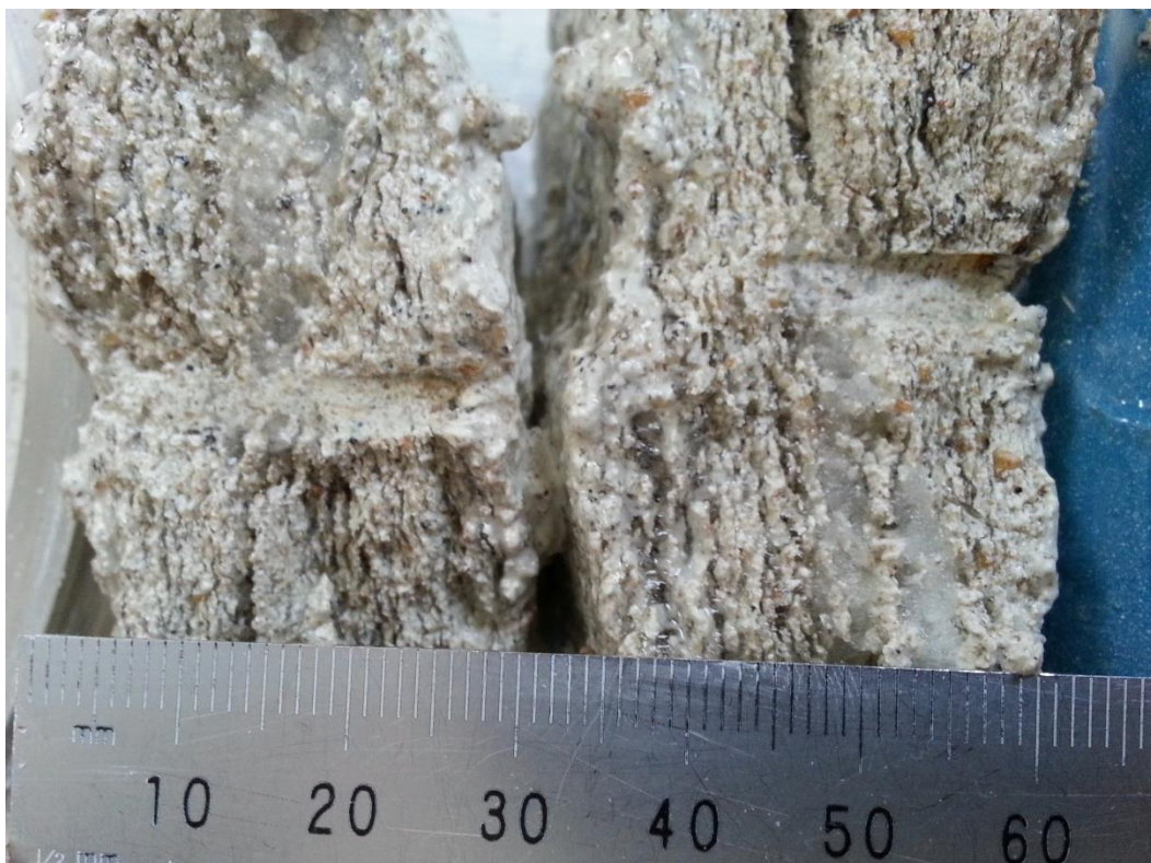
Figure 4.28 – Horizontal stratified structure of ice lenses at the top 10 cm layer of the sample supplied by deionised water for Test 1 (the sample is lying on its side)
