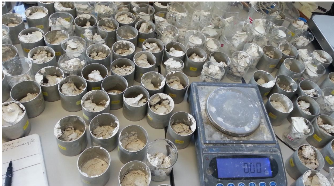
Fig 3.22 – Oven dried samples were used for chemical content determination
