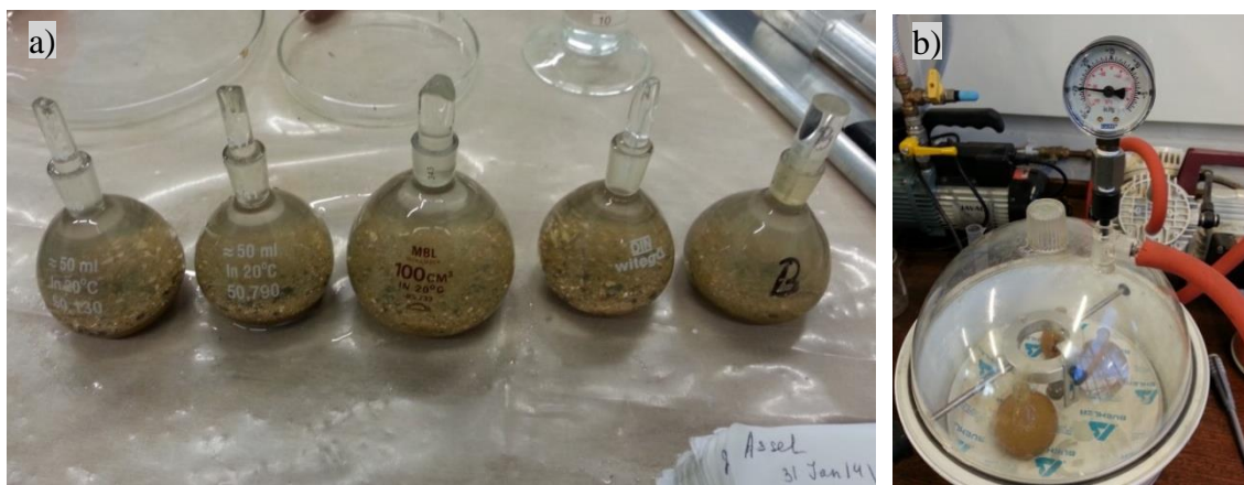
Figure 3.12 – Specific gravity test by the small pycnometer method:
