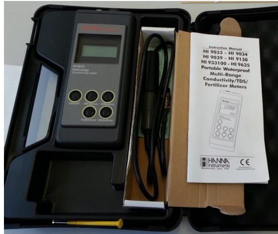
Figure 3.23 – Electrical conductivity meter for sodium chloride measurements
