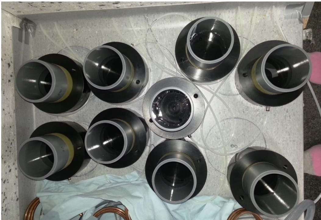
Fig 3.15 – Testing for leaks before assembling the mould
