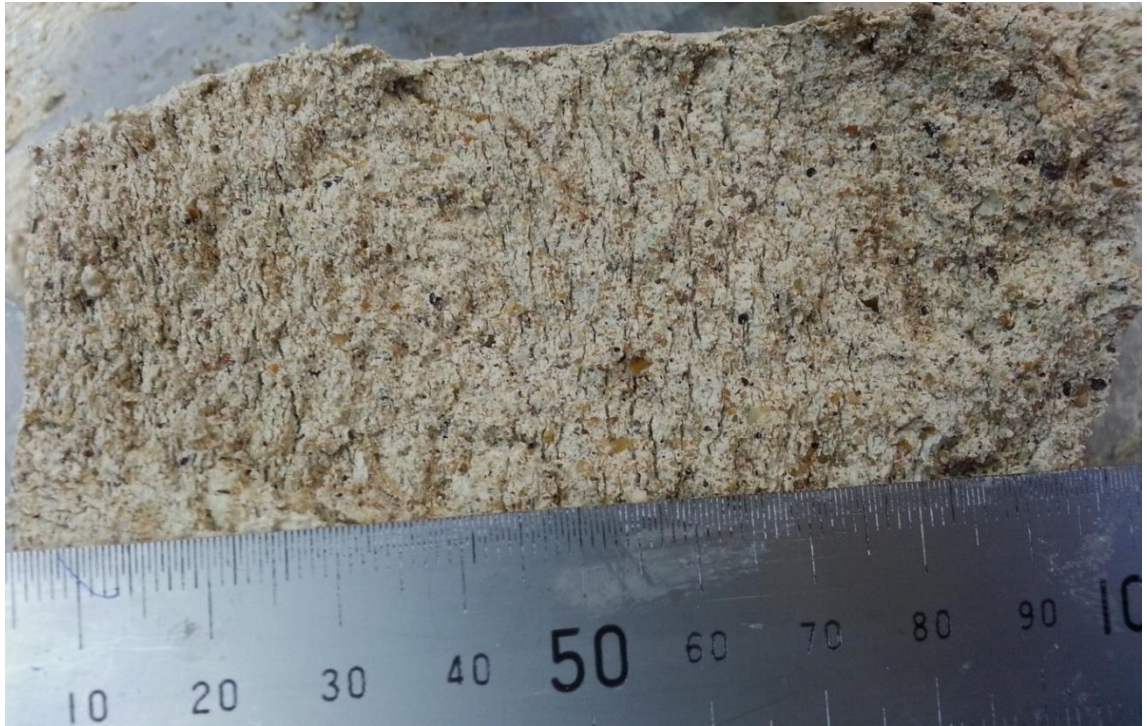
Figure 4.29 – Structure of the soil sample after freeze-thaw cycles supplied with 11,000 mg/l sodium chloride solution in Test 4 (the sample is lying on its side)
