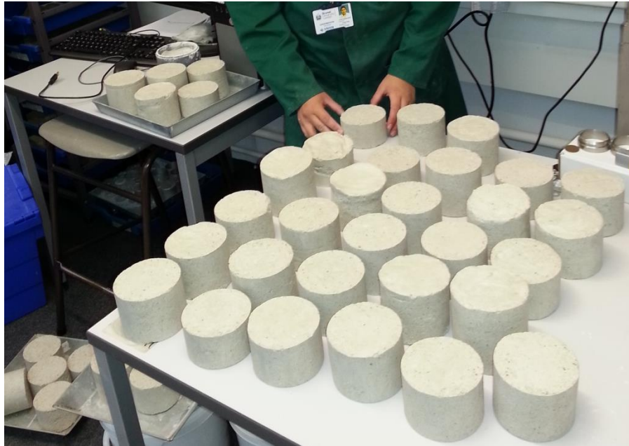
Figure 3.20 – Preparation of the remaining sample material for ultrasound testing
