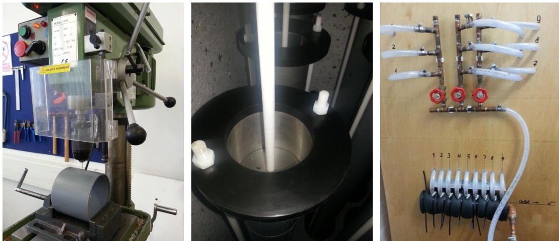
Figure 3.4 – Preparation of the experiment: a – perforation of a plastic mold for thermocouple insertion; b – surcharge sliding inside the chilling collar; c – cooling system control manifolds
