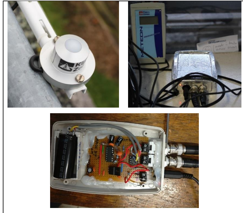
Figure 3.22. Pyranometer (irradiance meter) and signal amplifier
