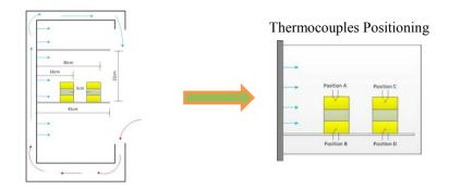
Fig. 5. Diagram of the experiment (side and front view)
