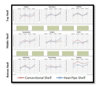
Fig. 6. Average temperatures of products placed on the heat pipe (blue line) and the conventional (red line) shelves for every position of the shelf
