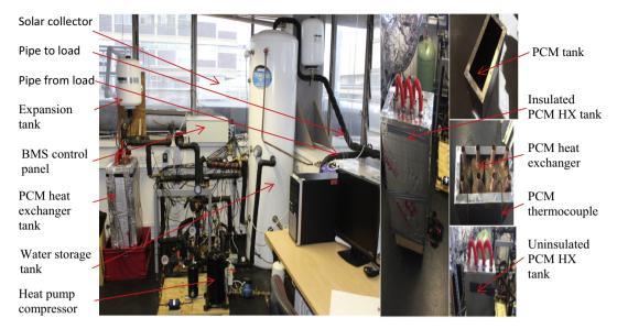
Fig. 2. PCM tank design and test rig setup.
