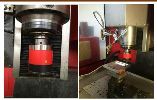
Figure 4-24: Infrared probe 32.00-MINI
