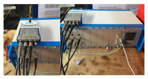
Figure 4-8: The data collection and multichannel change amplifier
