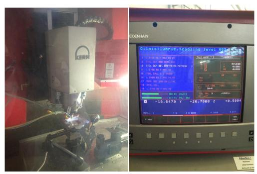
Figure 4-6: Drilling and monitor control
