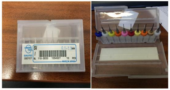
Figure 4-15: PCB Tungsten carbide drill tool
