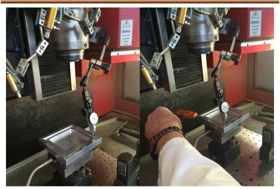
Figure 4-22: To calibrate the Aluminium fixture remains parallel to the moving direction of the base plate
