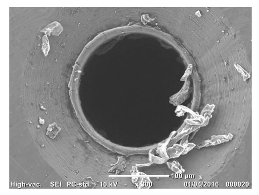
Figure 6-26:  $\Phi$  0.2mm drilled in Al work-piece entry side
