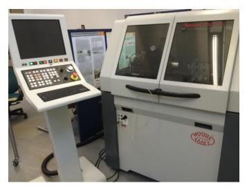
Figure 4-20: NANOTECH 250UPL Ultra-precision Lathe
