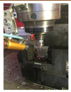
Figure 4-23: Laser tool position measuring system
