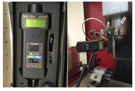
Figure 4-25: RS163-5348 Non-contact tachometer
