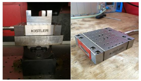
Figure 4-7: The Kistler dynamometer
