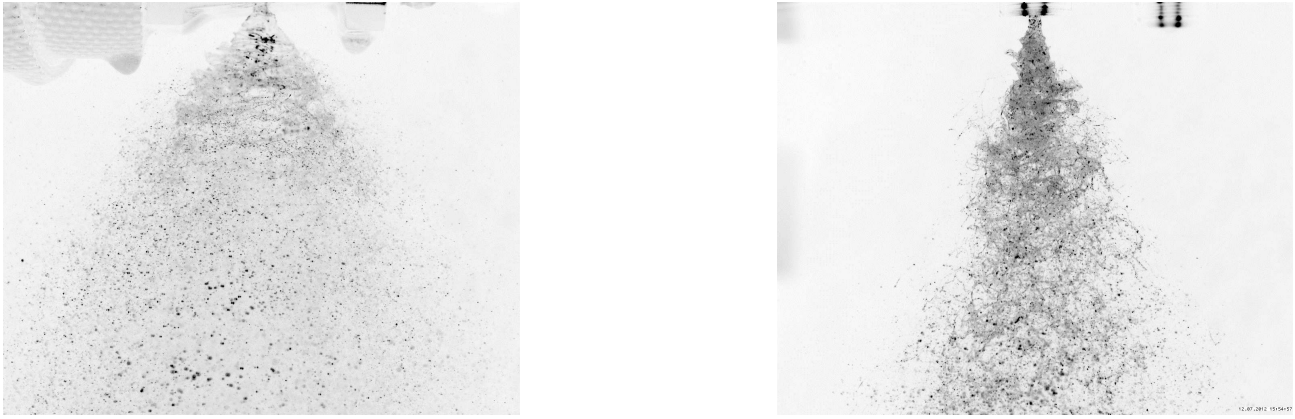
Fig. 2. Images taken with a high speed camera of two different types of nozzles (left: full-cone large angle; right: full-cone narrow angle) spraying oil at 80\text{ }^{\circ}\text{C} and 6\text{ bar}_g into an ambient reservoir
