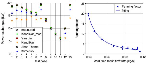
Figure 3: Model validation on thermal power Figure 4: Fanning factor calculated in test cases exchanged
