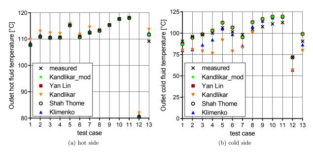
Figure 2: Comparison between measured outlet temperatures with model results obtained using different correlations for the phase change of the organic fluid
