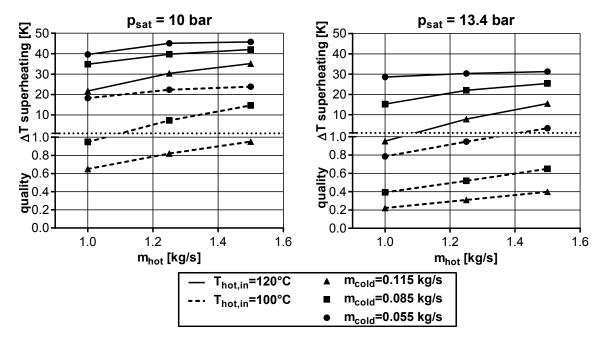
Figure 6: Effects of off-design operating conditions of a plate heat exchanger for waste heat recovery in terms of quality and superheating or subcooling of the organic fluid at the heat exchanger outlet
