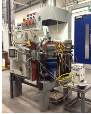
Figure 3.8 Photo of in-house built horizontal twin roll caster with integrated tundish and thermally controlled nozzle.
