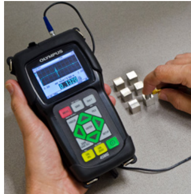
Figure 3.25 Elastic modulus measurement with ultrasonic thickness gauge (Olympus).
