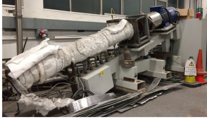
Figure 3.7 Photo of the twin-screw device for high shear treatment of Mg alloy.
