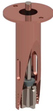
Figure 3.5 The schematic illustration of rotor-stator mixer for high shear treatment (Jiang 2013).
