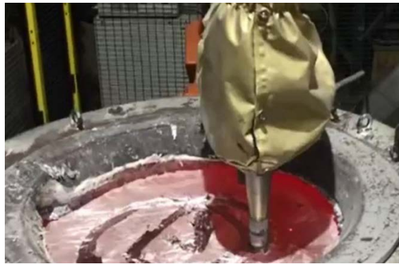
Fig. 5. Ultrasonic degassing prototype with a stepped sonotrode and a programmed movement enabled by a robotic arm [33].
