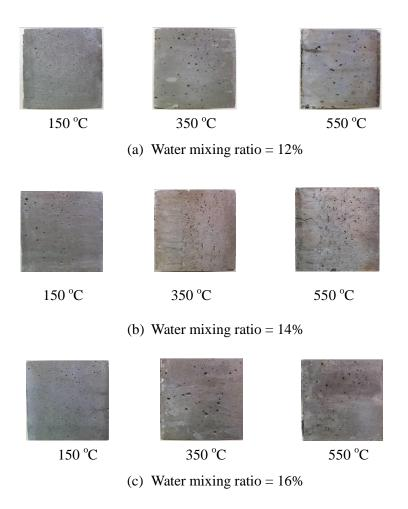
Fig. 1 Surface appearance of the specimens after heating.
