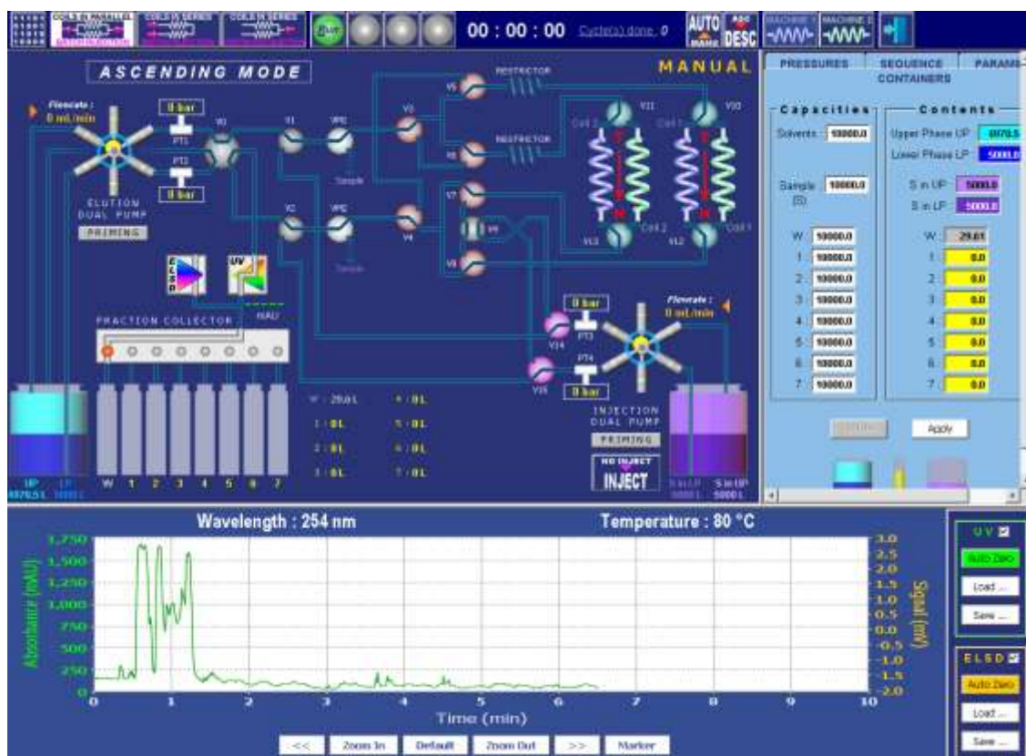
Figure 3.3: Armen Glider pumping system visual display for control of pumps, UV detector and fraction collector when operating the Maxi CCC instruments
