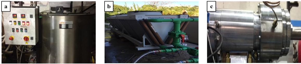
Fig. 2. Photographs of ORC system components (a) oil boiler and the controller; (b) cooling tower; (c) turboexpander.
