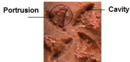
Figure 4.23: View of the treatment pattern (4.3 x 4.1) mm 2 , for Sample S1
