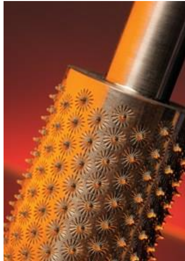
Figure 3.30: Laser Surface Treatment, (TWI, 2013).
