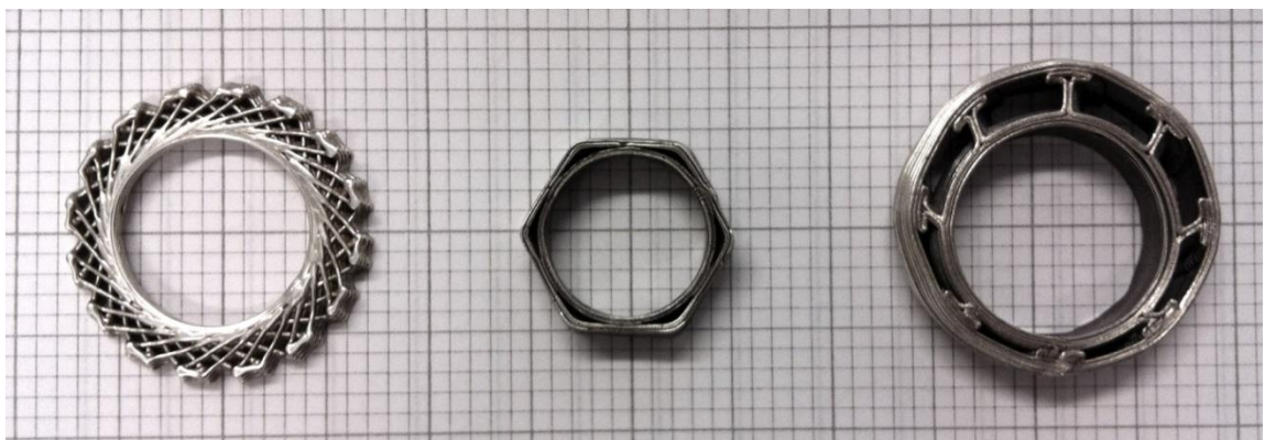
Figure 4.38. : Tessellation, Hex and Suspension structure comparison in 'PMC Pro'. figure by author
