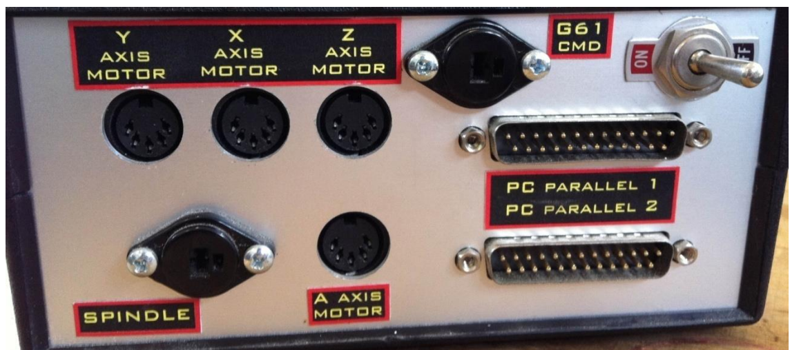
Figure 3.46, Sherline 5410 CNC mill controller. figure by author
