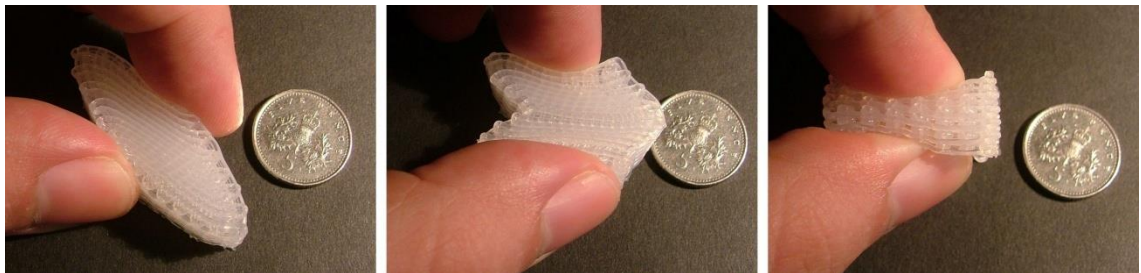
Figure 3.18, 23.6mm 2 x 13 layer build, behaviour when compressed at 45°(left) , 90° (middle) and along the Z axis. figure by author
