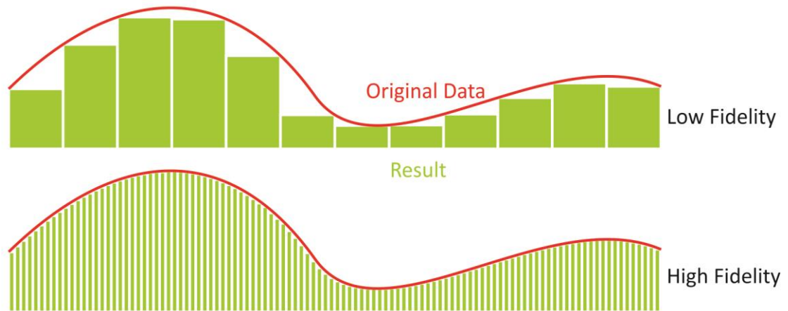
Figure 2.70, Mp3/build fidelity comparison, thick bars indicate thicker layers. figure by author
