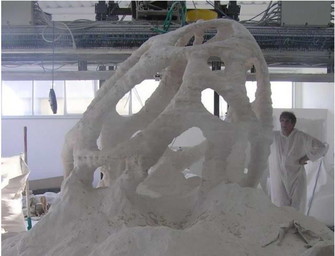
Figure 2.44, large print "radiolaria" made on D-shape system during the 'evaluation process' (D-shape, n.d.)
