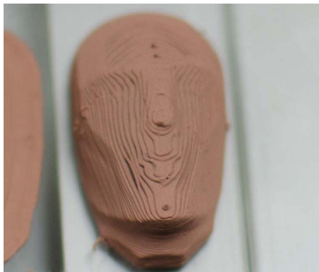
Figure 5.5, 15mm vertical length, 0.17mm layers. BronzClay. figure by author
