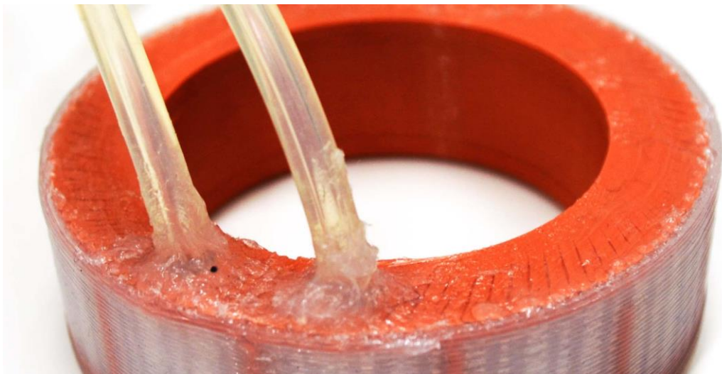
Figure 4.14, Finished thermal cuff with inlet and outlet tubes installed. figure by author
