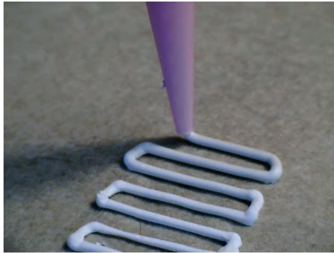
Figure 3.27, PMC3 line deposition test on grease paper. figure by author
