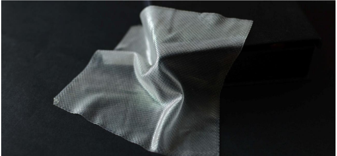
Figure 4.1, Silicone textile made with 0.2mm nozzle. figure by author
