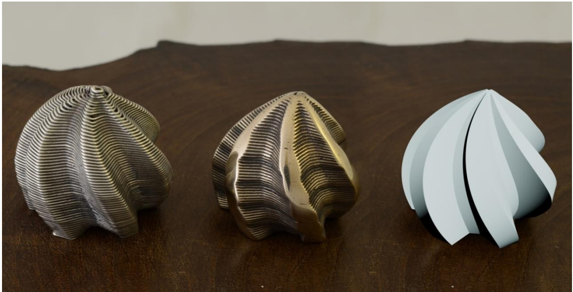
Figure 4.31, Seashell in 'PMC Pro', 'BronzClay' and CAD geometry. figure by author
