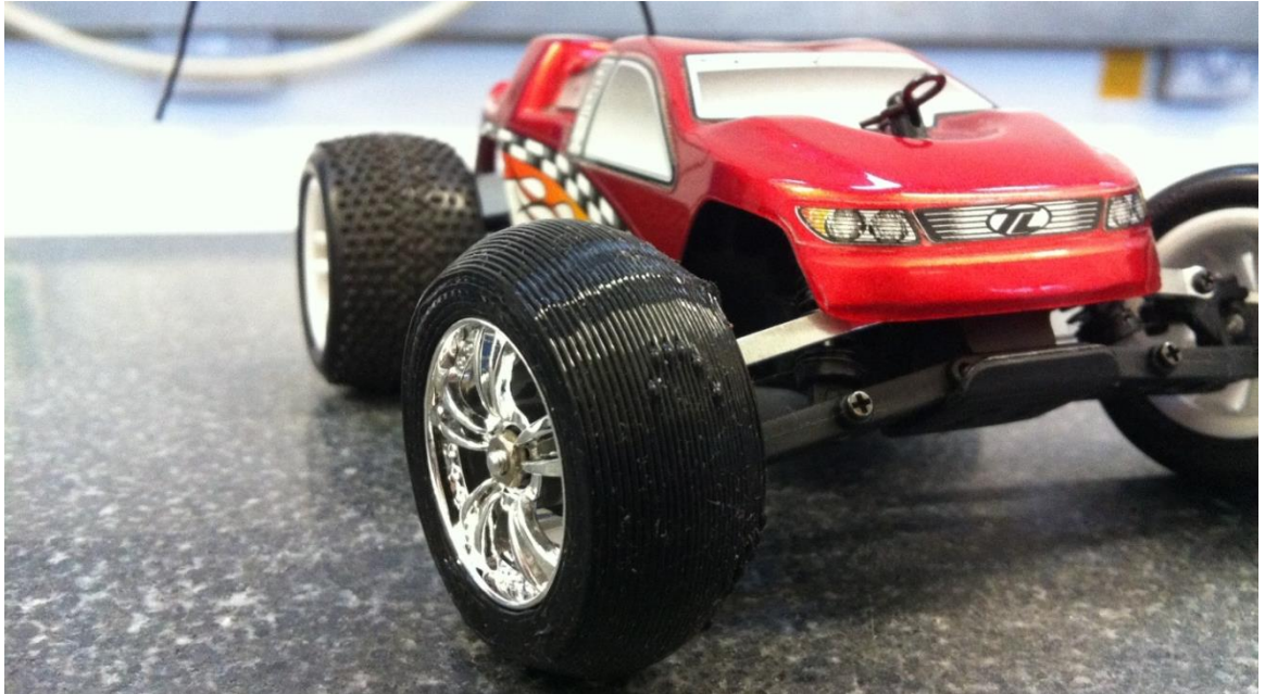
Figure 4.25, RC car with silicone tyres fitted. figure by author
