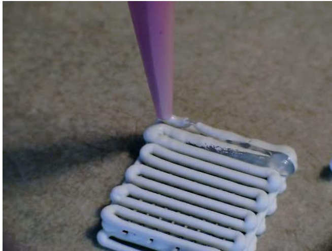
Figure 3.29, Final PMC3 periodic structure sample #6, silicone was used to flush the remaining material inside the nozzle as can be seen in the last three filaments. figure by author
