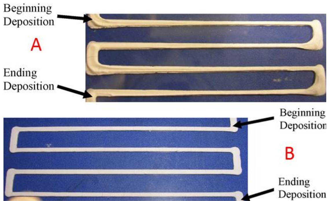
Figure 2.58, Track deposition test. A: constant ram velocity. B: Extrusion force controller. figure by Mason (2009, p.2954)
