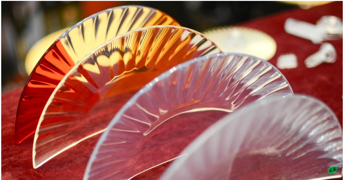
Figure 2.18, finishing grades on SLA parts, made by Malcom Nicholls, figure by author.
