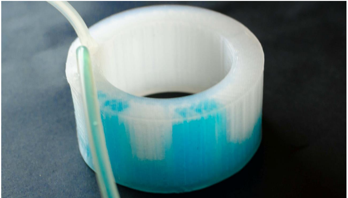
Figure 4.16, Revised thermal cuff with blue liquid flowing through it. figure by author
