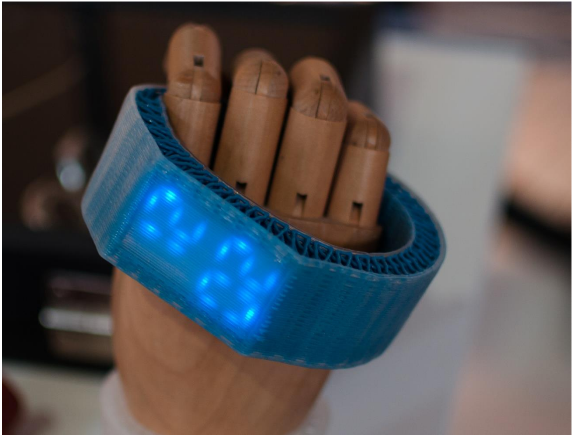
Figure 4.8, Complete AM watch in blue and clear silicone. figure by author
