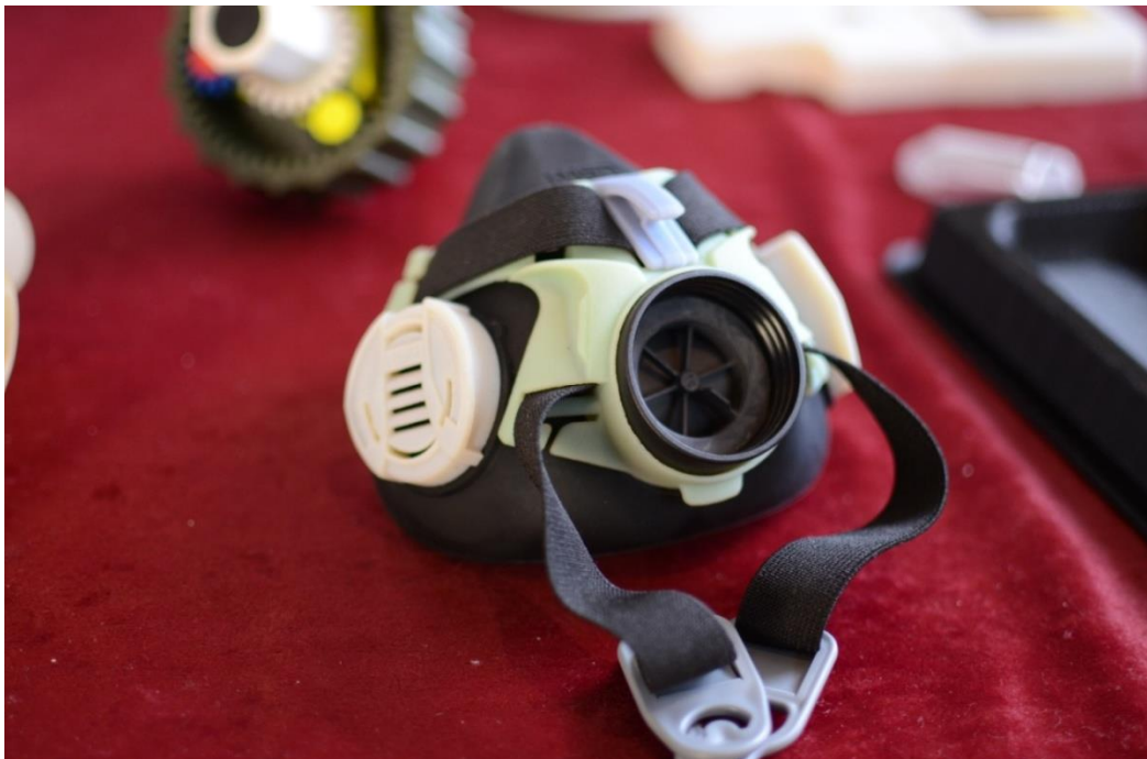
Figure 2.32, Object printed on Objet system with rigid and flexible materials. figure by author
