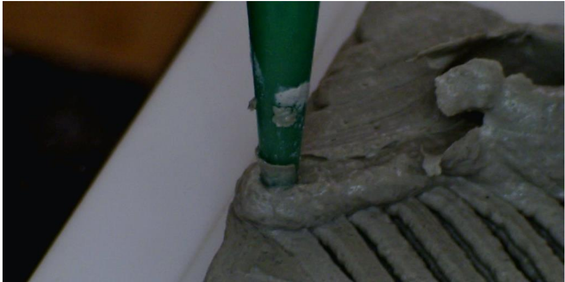
Figure 3.60, Deposition with Nylon reinforced clay, 0.8mm nozzle, moment the build failed. figure by author
