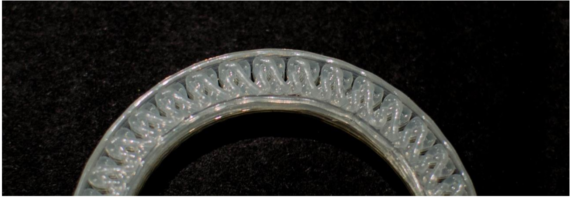
Figure 3.80, Build with 1.2mm nozzle showing the defects at the outer edges of the spokes. figure by author
