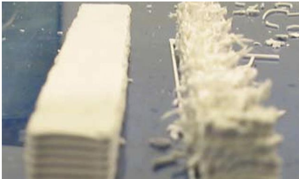
Figure 2.59, Side view of Al 2 O 3 bars fabricated using extrusion force controller (left) and constant ram velocity (right, v = 2 m/s). Table speed is 19 mm/s, standoff distance is 0.5mm, horizontal line shifts are 0.5mm, and nozzle diameter is 580micron.
