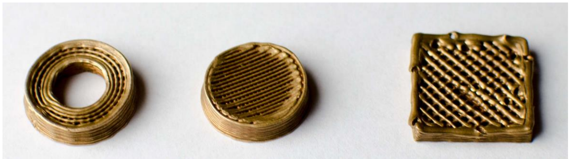
Figure 3.116, Fired test samples 1, 2 and 3. In BronzClay. figure by author
