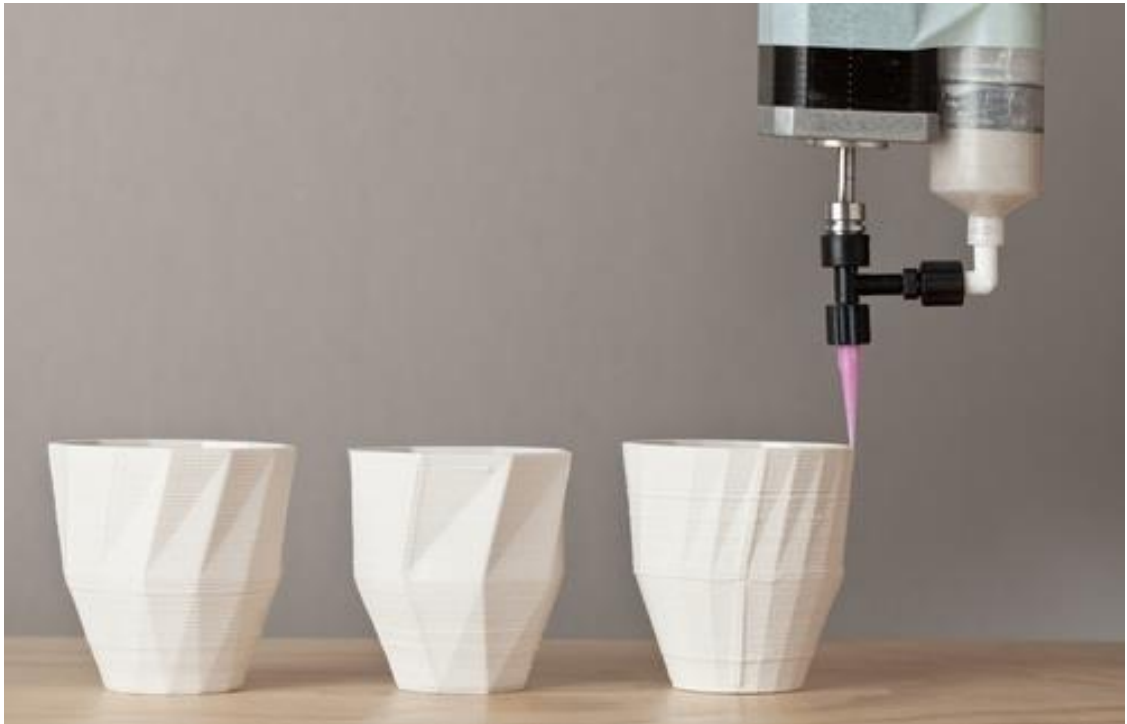
Figure 2.38 Unfold ceramic printer, porcelain cup. photo by Kristof Vrancken (unfoldfab, 2012).
