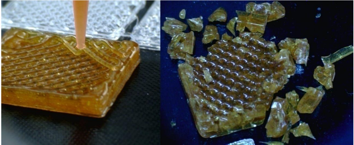
Figure 3.58, Left: deposition of Dextrin with Mk3, Right: explosive structural failure of Dextrin while drying. figure by author
