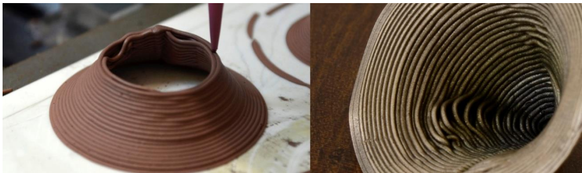
Figure 4.28, 40° cone deposition defects . figure by author
