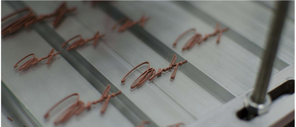
Figure 5.4, Improved resolution demonstration, BronzClay. figure by author
