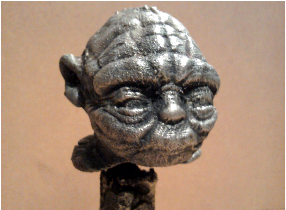
Figure 2.12, Rob Bryan's Lost PLA cast aluminium Yoda bust, partial casting. (Bryan, 2012)
