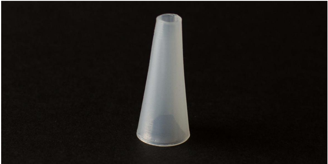
Figure 3.101, G-code cone test, 17mm diameter at the base, 0.4mm nozzle, 0.35mm layers. figure by author
