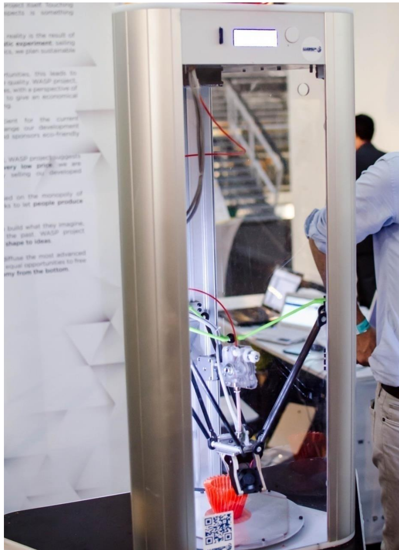
Figure 2.6, Delta FFF system manufactured by WASP, figure by author
