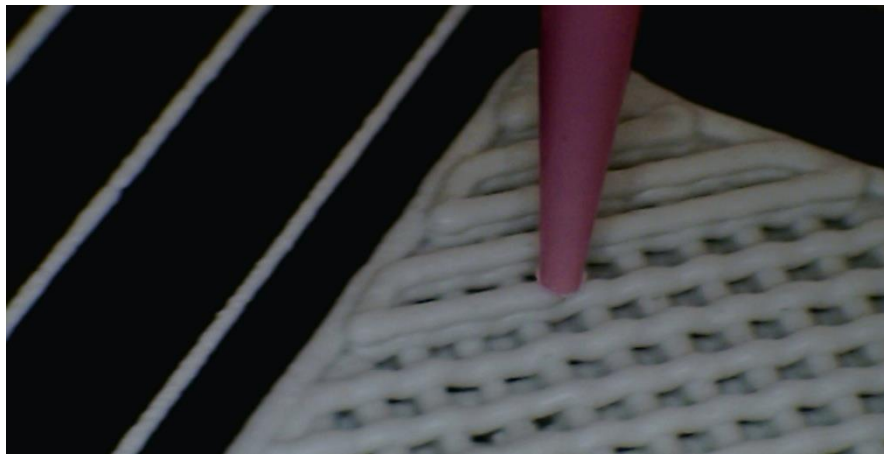
Figure 3.57, Deposition of two layers of the same pattern, improved filament quality. Material: Talc + PVA. figure by author
