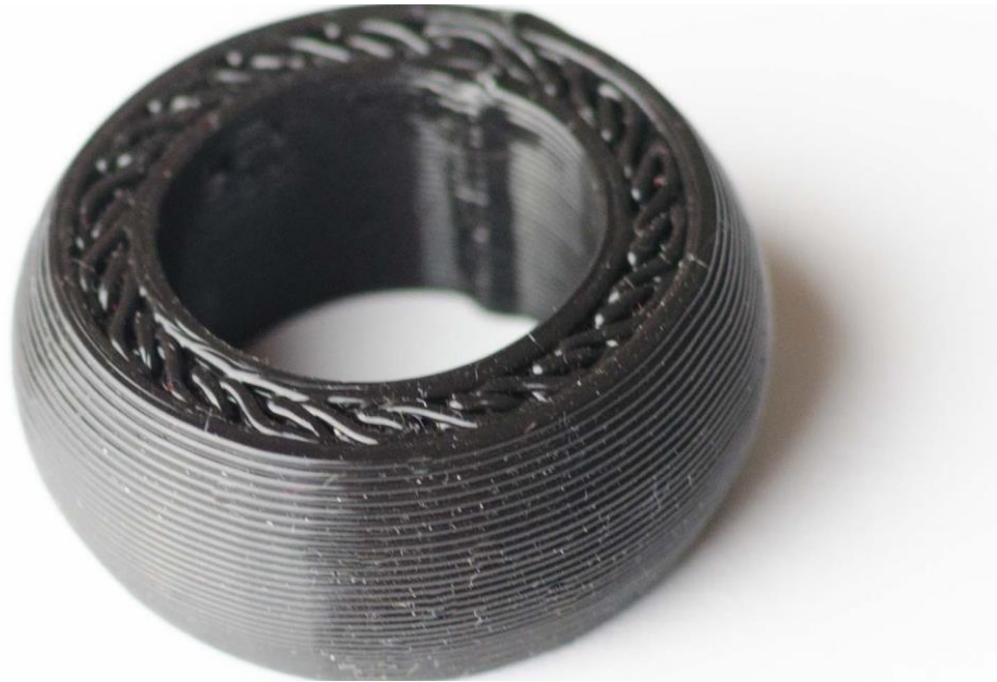
Figure 4.24, RC car tyre made with the 2D+3D method and the tessellated infill. figure by author
