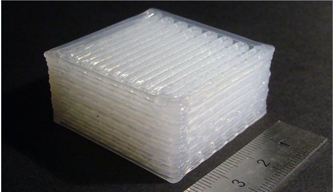
Figure 3.43, 16 layer build with Mk2 equipment. figure by author
