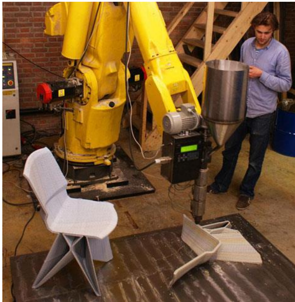
Figure 2.45, Endless chair being built. figure by Endless. (Kennedy, 2011)
