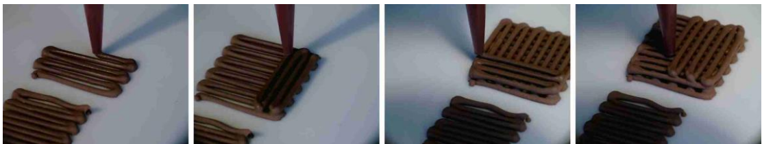
Figure 3.34, The process of depositing a four layer sample. BronzClay, 0.6mm nozzle, 2.1 bar pressure. figure by author
