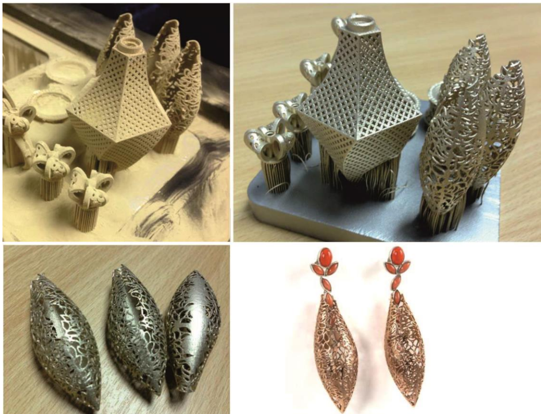
Figure 2.24, work piece just after the build is complete and loose powder brushed off (top left). Work pieces cleaned and shot peened (top right). Support removed (bottom left). And final piece polished (bottom right). Bottom piece designed and finished by Charlotte Parkhill 2013, images courtesy of estechnology (Cater, 2013)
