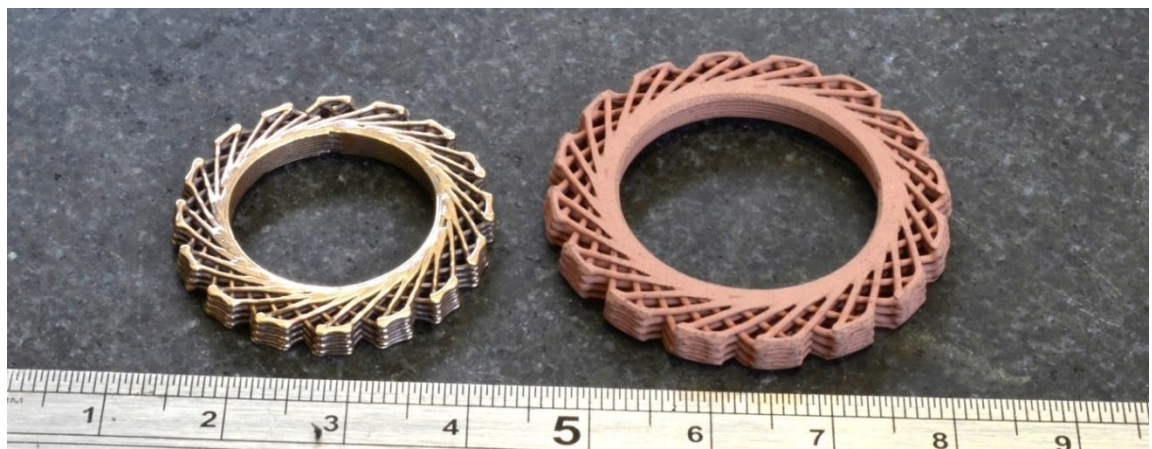
Figure 4.33, Tessellated ring design pictured in both its greenware state and fired state. figure by author
