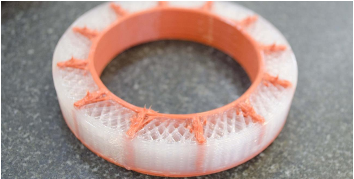
Figure 4.11, Partially completed thermal cuff showing spokes used to direct the flow of water (orange). figure by author
