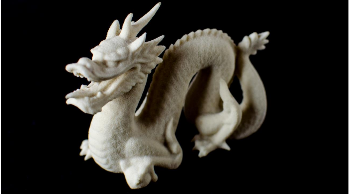
Figure 2.29, Dragon made with Voxeljet system, material: PMMA with Polypor B binder for investment casting. figure by author
