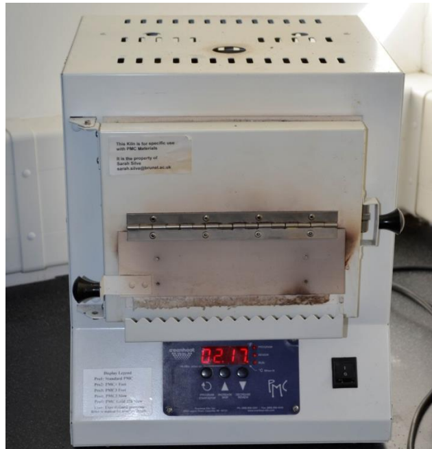
Figure 3.30, PMC Kiln, Even Heat 360. figure by author
