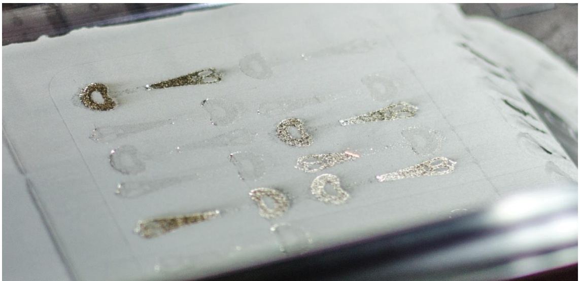
Figure 2.20, LaserCusing process building small spoons in silver, note the laser beam in the middle/right section of the image. figure by author.
