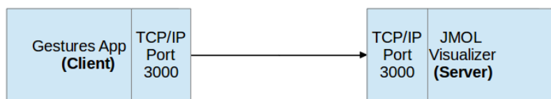
Figure 4-8: Communication between the GestureApp and other modules.
