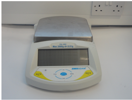
Figure 3–1 Adam Equipment PGL 2002 Precision Balance used in measuring the mass of food items and their waste products
