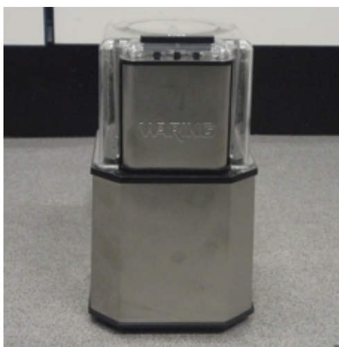
Figure 3–11 Waring High Performance grinder used for milling of food waste samples
