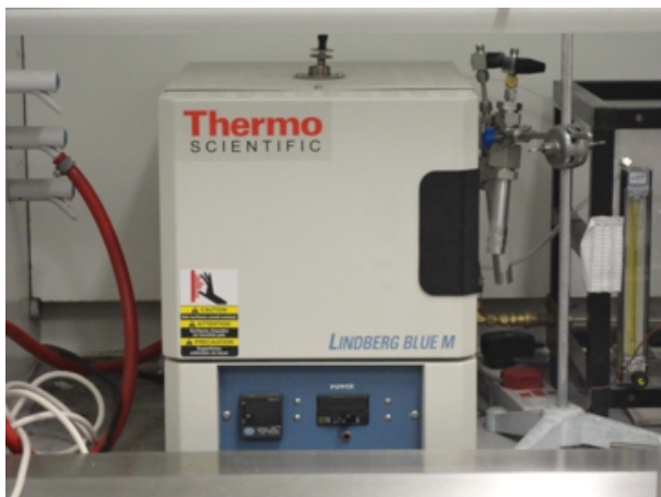
Figure 3–10 Thermo Scientific box furnace used for drying of food waste samples
