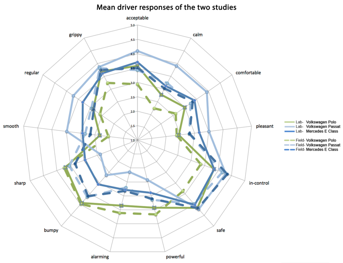
Figure 7.10 The Semantic Space showing a comparison of each automobiles activation pattern measured in the field study and the laboratory test bench
