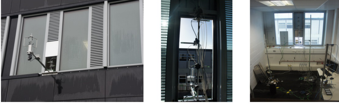
Figure 5: Instrument set up. Left: 3D Ultrasonic anemometer measuring boundary conditions. Middle: Typical opening case with E+E thin film anemometers measuring velocity. Right: internal layout and test room set up
