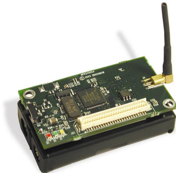
Figure 2.1: Berkeley mote (MICAz MPR 2400)
