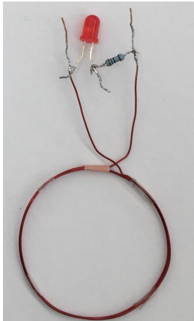
Figure 4.6: Load coil with load resistance R_L and LED's
