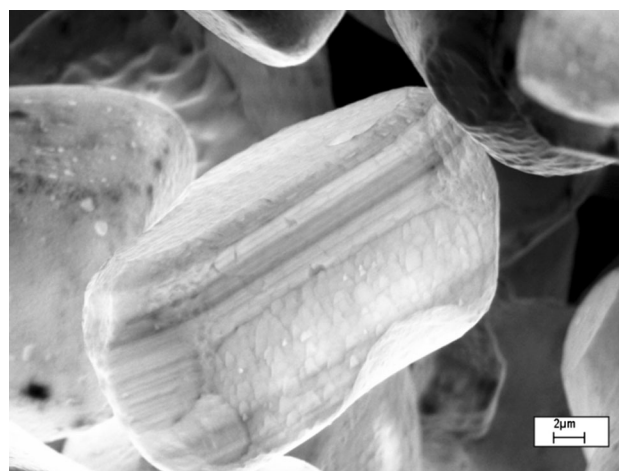
Fig. 3 CL image of ACEL phosphor particles
