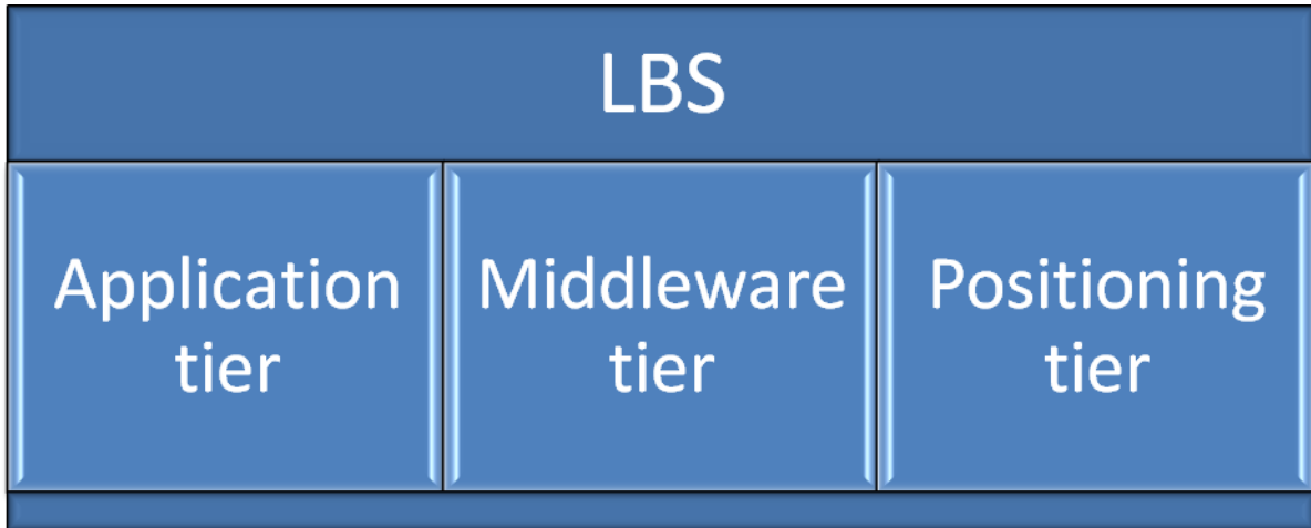
Figure 2. 5: Location-based service (LBS) architecture (Schiller and Voisard, 2004)
