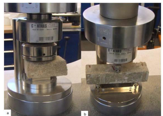
Figure 3.8: Strength testing INSTRON jig for compression and flexural test
