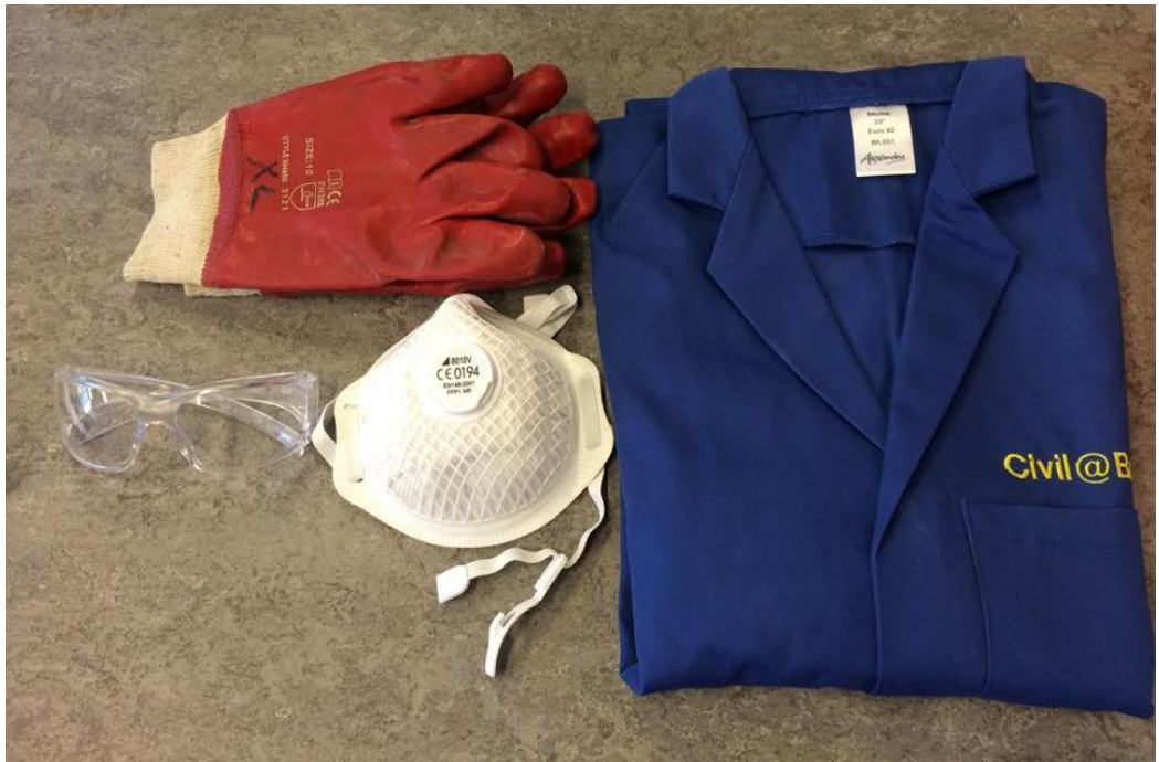
Figure A: list of PPE (Gloves, Lab Coat, Breathing mask and safety glasses)
