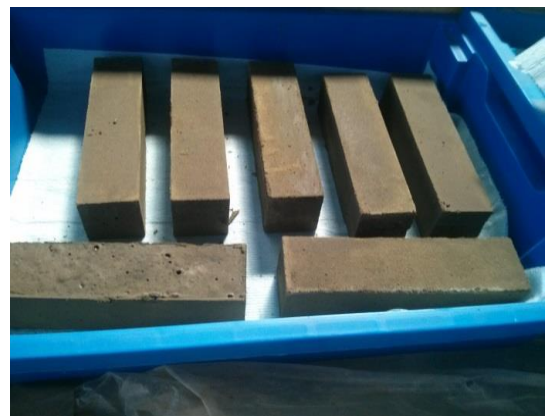
Figure 3.6: Sample preparation for curing at 20^{\circ}\text{C}
