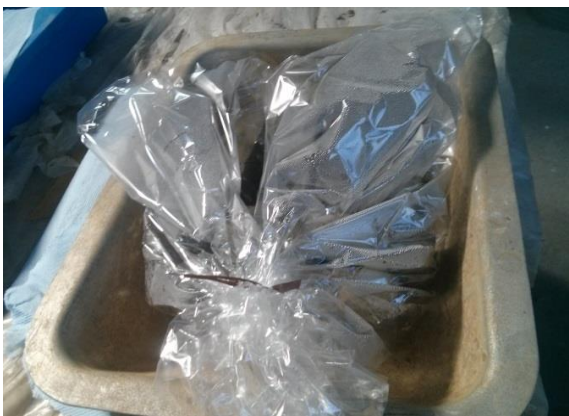
Figure 3.7: Sample preparation for curing at 70^{\circ}\text{C}
