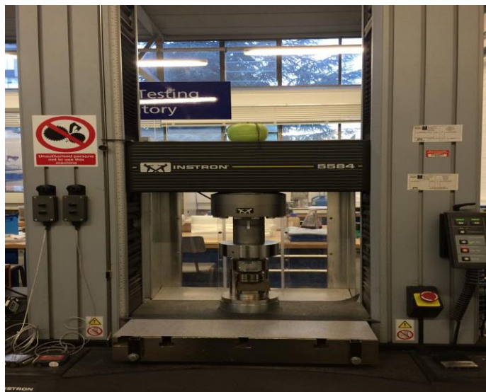
Figure 3.10: INSTRON 5584 System used for sample Compressive test
