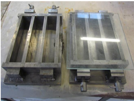
Figure 3.5: ELE prismatic moulds 40x40x160 mm 3
