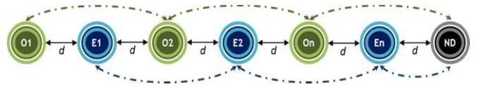
Fig. 3: A dual path linear topology with O_n/E_n number of source nodes and ND as destination node evenly distributed in d within half the communication range.
