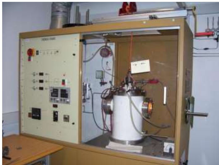
Figure 3.2. HFCVD reactor used for diamond coating deposition (P. May, 2012)
