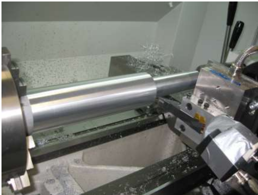
Figure 3.10. Instrumented lathe setup for cutting trials.
