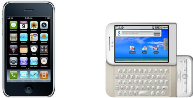
Fig. 1.1 - iPhone (first model) (left) and HTC Dream, first device running Android (right)
