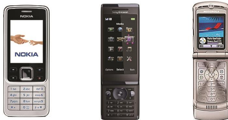
Fig. 6.4 – Different handset models portraying innovative form factor. From left to right: Nokia (candy bar); Sony Ericsson (slide) and Motorola (clamshell).
