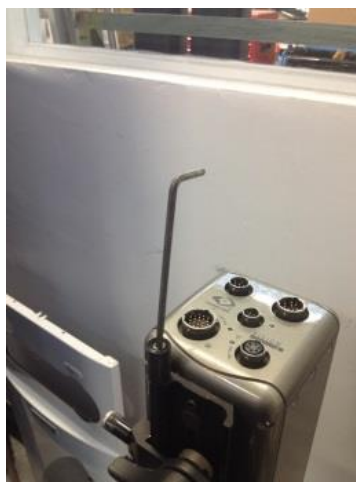
Appendix 36. Allen key used to move the camera with 0.3125 mm intervals.
