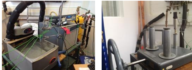
Figure 3-18. Water bath (left) and dead weight tester (right).
