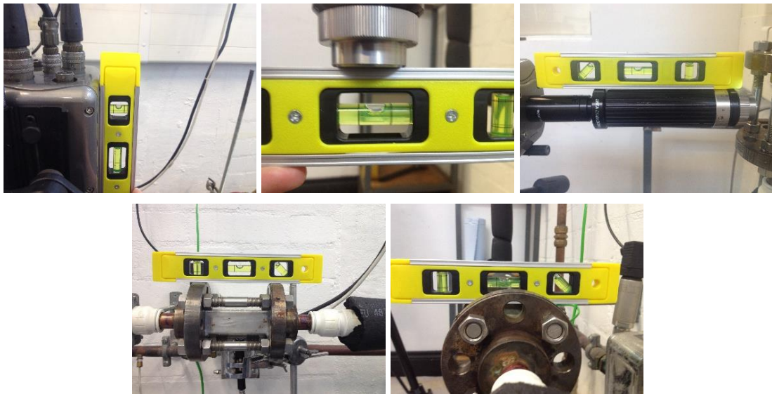
Appendix 21. A level ruler used to verify axes of camera setup and sight glasses.
