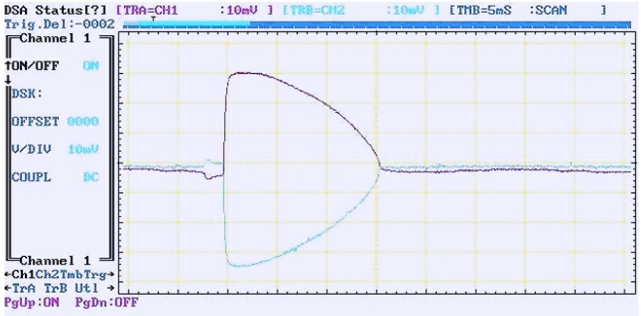
Figure 1. Initial event: peak voltages; drop -2.3\text{mV} ; plane surface 2.3\text{mV} . Event duration, 2.4\text{ms} .
