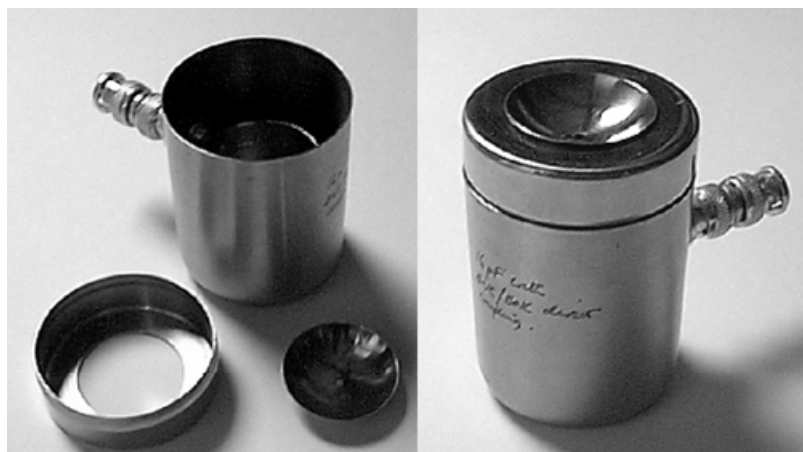
Figure 5.3. Faraday Cup, dismantled ( left ) and assembled ( right ).
