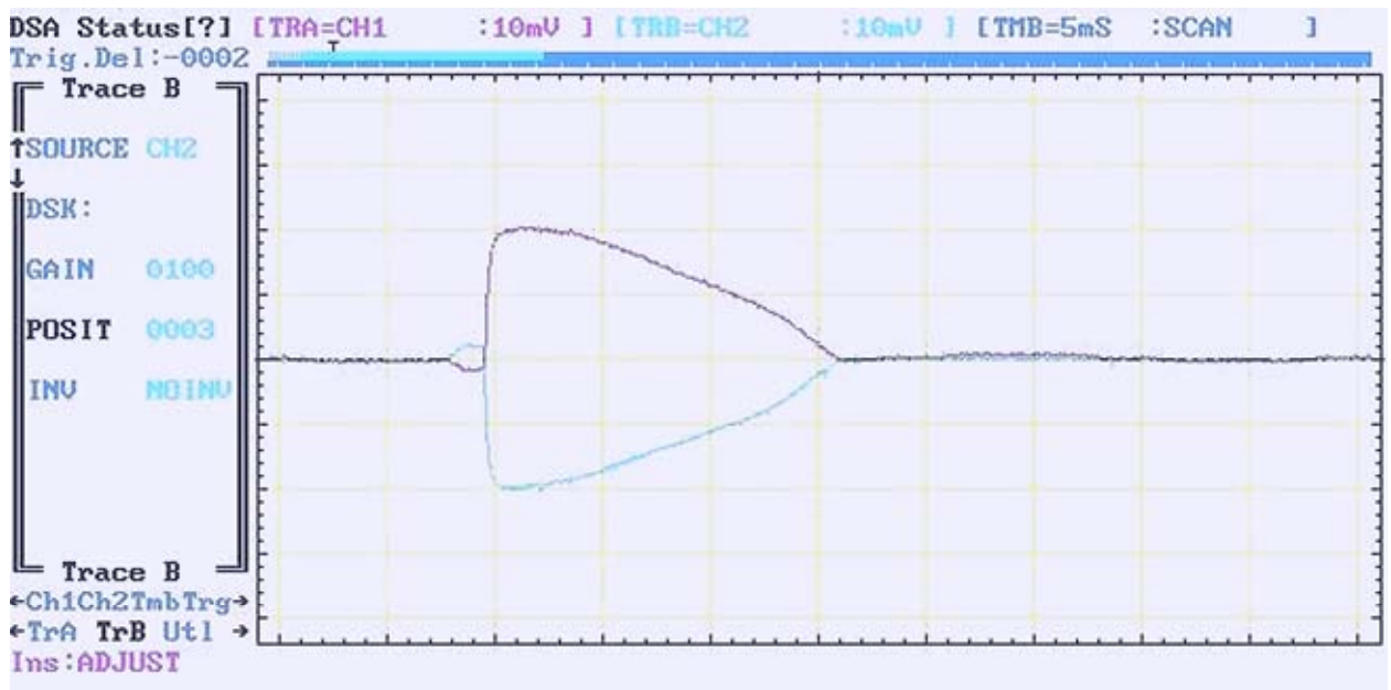
Figure 4. Initial event: peak voltages; drop -1.8\text{mV} ; plane surface 2.2\text{mV} . Event duration, 1.9\text{ms} .
