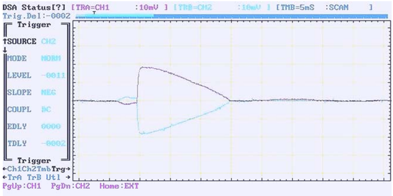
Figure 7. Initial event: peak voltages; drop -1.2\text{mV} ; plane surface 1.2\text{mV} . Event duration, 3.7\text{ms} .
