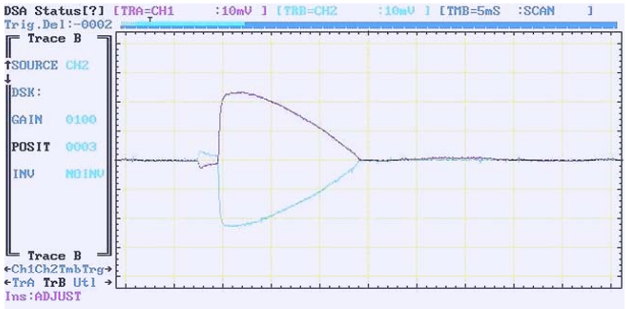
Figure 3. Initial event: peak voltages; drop -3.0\text{mV} ; plane surface 3.0\text{mV} . Event duration, 2.3\text{ms} .
