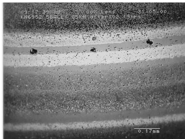
Fig. 10 No 2 ball after 102 hours 19 minutes 5-ball rolling test
