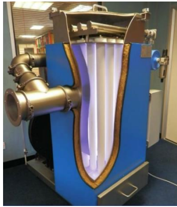
Figure 3-7: Hot gas ceramic filter module (Glosfume, 2013).
