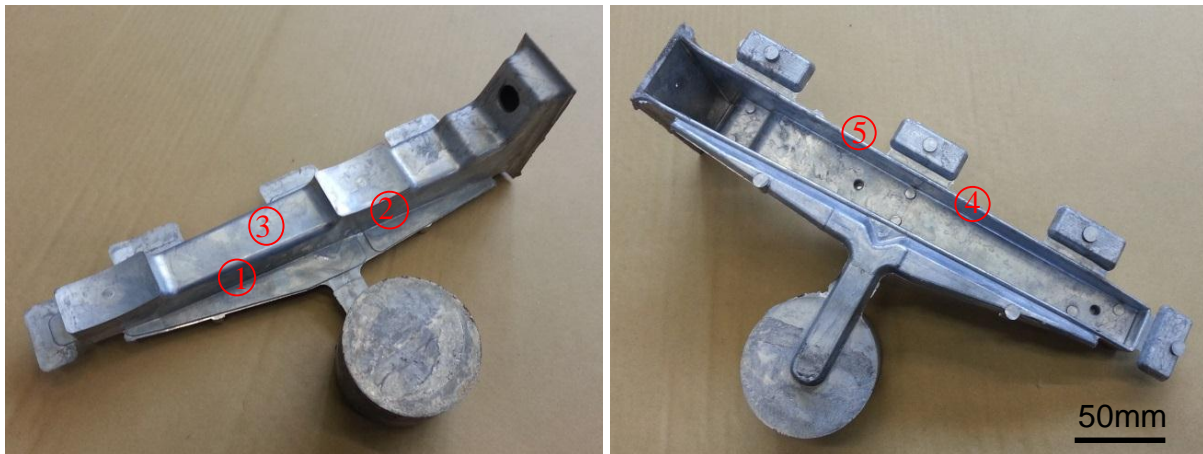
Figure 8.42 The photos showing the casting structure with runner, over flow and biscuit for evaluation of the reproductivity.
