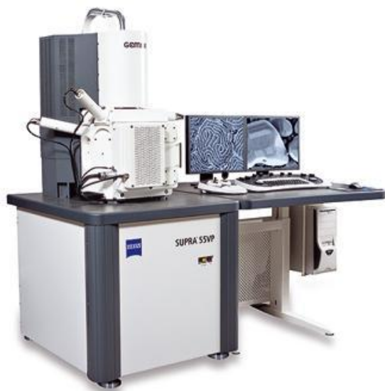
Figure 3.13 The photo of Zeiss Supera 35 FEG scanning electron microscope (SEM) equipped with an energy dispersive X-ray spectrometer (EDX) facility.
