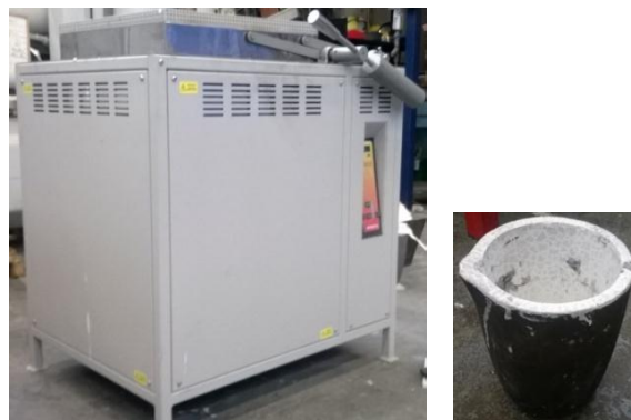
Figure 3.1 The photo of the electric resistance furnace and the clay-graphite crucible used in the current study.
