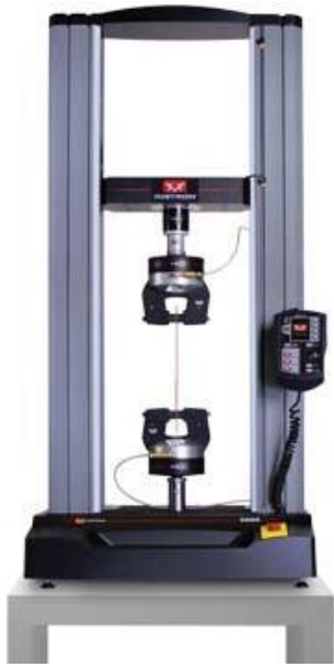
Figure 3.15 The photo of Instron ® 5569 universal materials testing machine.
