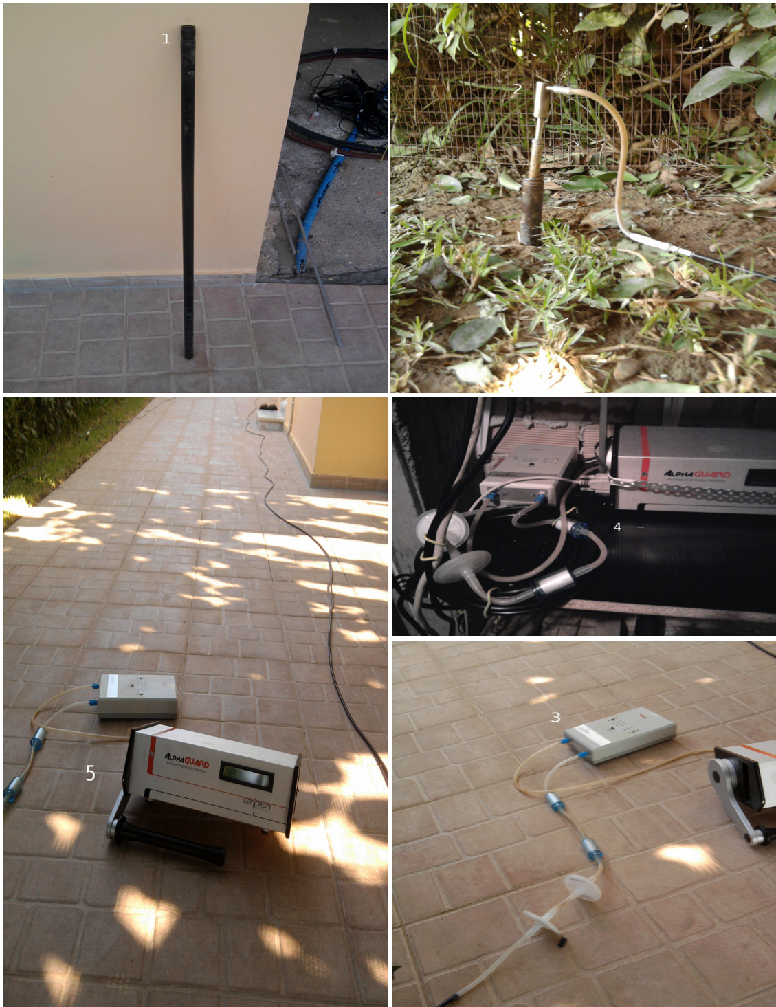
Figure 3.12: Ileia: a) Probe (1,2) b) Alpha Pump and accompanying equipment (3,4,5) c) Alpha Guard (4,5).
