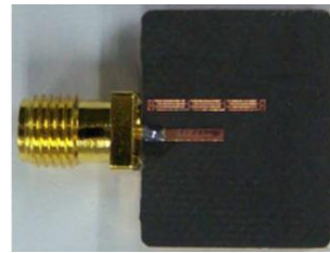
Fig. 1-18. Dual-band MZR antenna, (a) perspective view (b) fabricated prototype [70]
