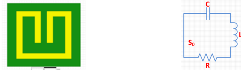
Fig. 2-2. SRR structure and its equivalent resonant circuit
