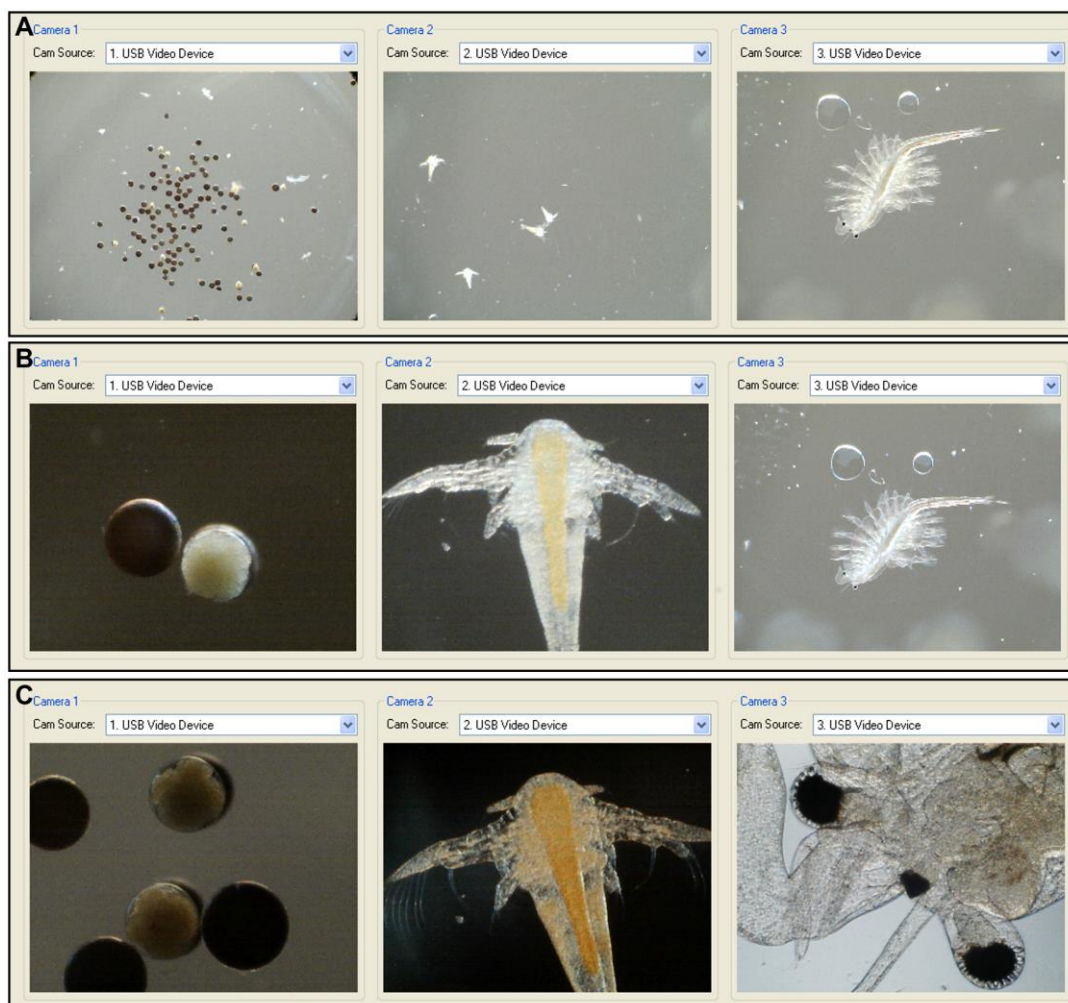
Figure 6.11. Screenshot of Autokams which demonstrates the ability of the microscope system to image distinct samples in different manners simultaneously. A) Cyst, nauplii and adult Artemia at 15.76x magnification B) Cyst and nauplii at 206.86x, adult at 15.76x C) All three stages at 206.86x magnification.
