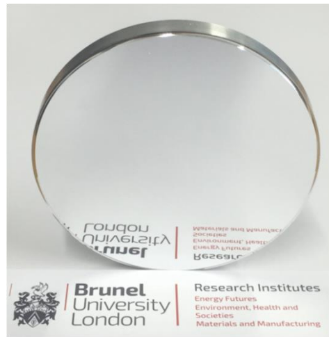
Figure 6.12: Example of workpiece manufactured by the smart cutting tool
