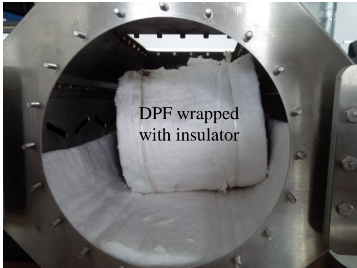
Figure 8.9 Non-catalysed DPF inside the MW cavity
