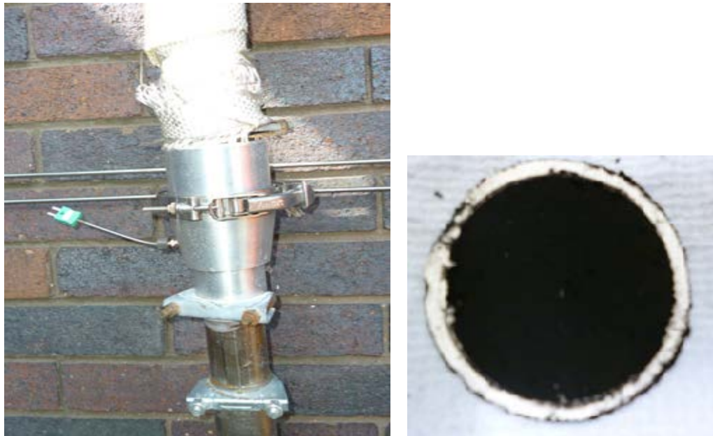
Figure 7.1, A: Cartridge holder modified on line, B: Filter element loaded with soot
