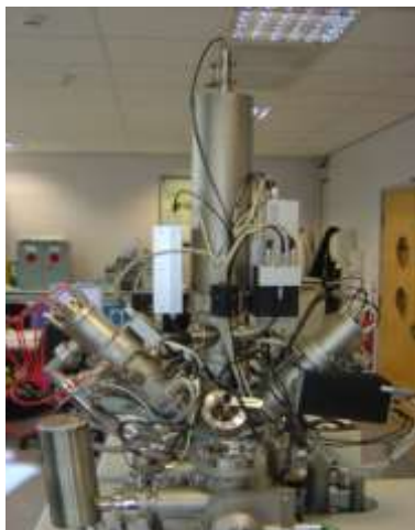
Figure 3.24: The ToF-SIMS instrument, known as ION-TOF-GmbH used for the surface chemical group characterization of adhesive films.
