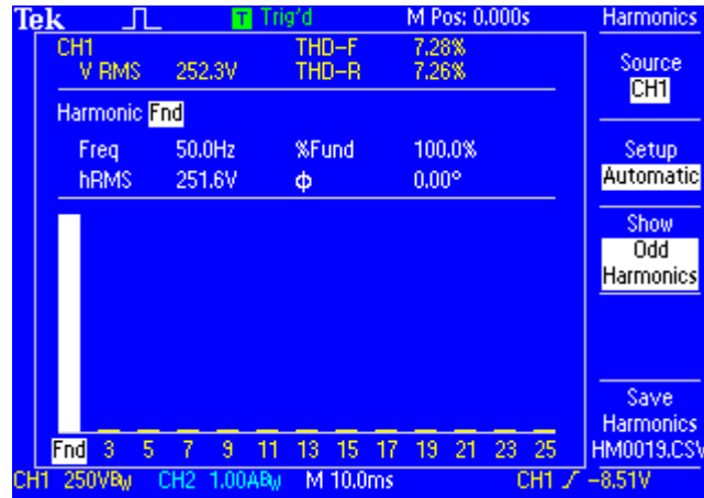
Fig. 6-5 FFT of output voltage of BBLFI circuit in case study 2.
