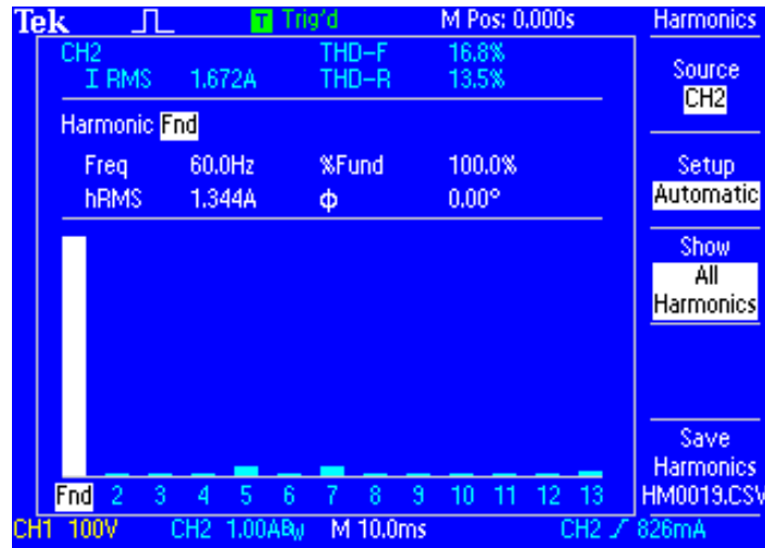
Fig. 6-13 FFT of output current of FLFI circuit
