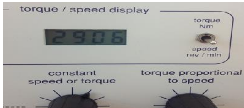
Fig. 6-15 The control torque panel of induction motor
