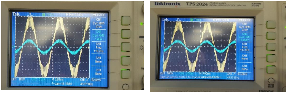
Output current and output voltage of FLFI circuit with 118Hz and 117Hz output frequency
