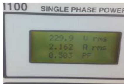
Fig. 6-16 voltage across of load, current of load, Power factor of induction motor
