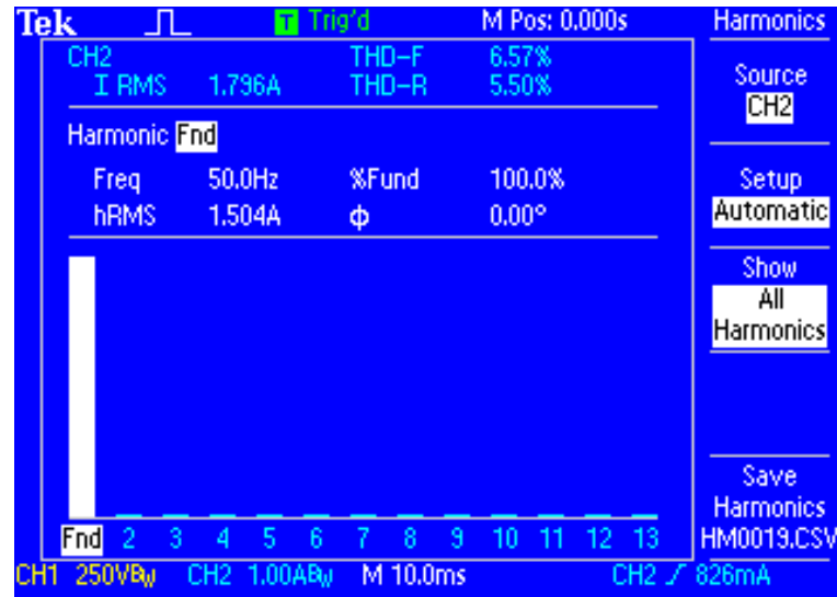
Fig. 6-10 FFT of optimised output current of proposed circuit
