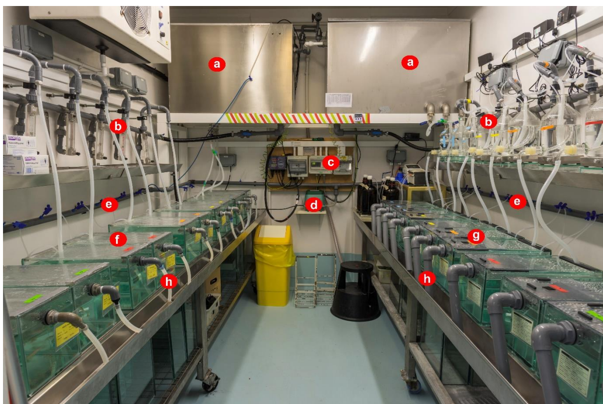
Figure 23: Adult zebrafish 14-day exposure room setup. (a) Header tanks containing carbon filtered mains tap water feeding to (b) individual flow meters and tank feeds. (c) Temperature controls for header tanks. (d) Air pump leading to (e) individual tank air feeds. (f) Pre-study 7-day acclimatisation tanks. (g) 14-day exposure tanks. (h) Individual tank out flows, draining to mains sewerage system.
