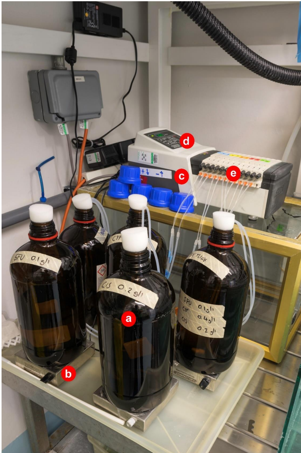
Figure 24: Delivery system for drug dosing. (a) 2.5L brown glass (to reduce photolysis of drug) bottles with foam stoppers to reduce evaporation and hold tubing in place. This photograph was taken during the mixtures experiment, so the stock bottle on the right contains the three drugs at the same concentration as their individual stocks. In each experiment the control tanks were dosed with ddH 2 O (stock bottle back left). All replicates at a given concentration and control are fed from one dosing stock bottle. (b) Each stock bottle sits on a magnetic stirrer and the stock solution is kept in motion with a magnetic stirrer bar, to prevent the drug from coming out of solution. (c) The stock solutions are fed to the mixing vessels via a peristaltic pump. This works by massaging narrower gauge tubing with rollers rotating in the direction of flow. This keeps the stock solution within a “closed” circuit, reducing the chance of both cross contamination of dosing stocks and contamination of pumping equipment. (d) Control panel for setting rotation rate for approximate dosing rate. (e) Individual adjustment knobs to fine tune flow rate to each exposure tank. Further tubing (not visible above) continues to individual mixing vessels (Figure 25).
