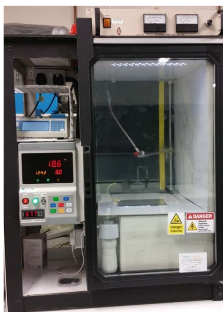
Figure 3.3: In-house electrospinning box produced with the help of AC solutions.
