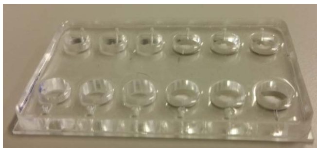
Figure 3.6: Fabricated open chamber PDMS cartridge for 1064nm Raman testing
