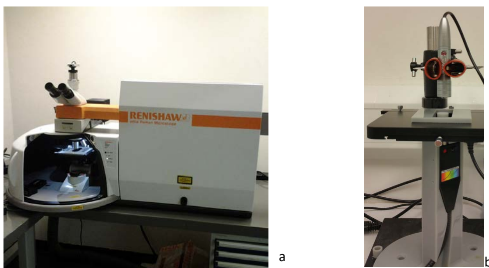
Figure 3.5: Image a) shows the 514nm InVia Raman set-up from Renishaw, b) shows the 1064nm portable Raman probe set-up by Stellarnet in modified 3D printed platform.
