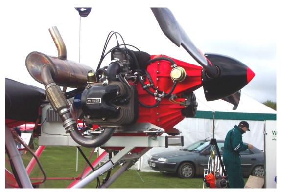
Figure 5, Verner 133M Engine fitted to X'Air 'F' Aircraft
