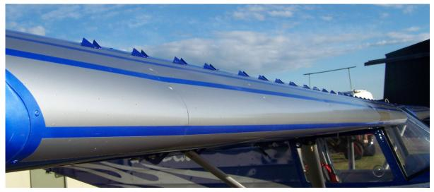
Figure 3, Savannah VG leading edge vortex generators
