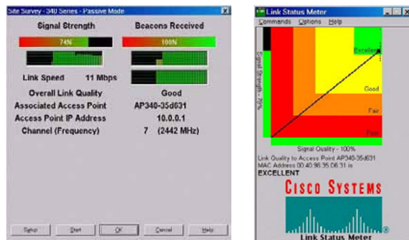
Fig. 4.12 Site survey tools provided by Cisco systems indicate signal strength and signal quality.
