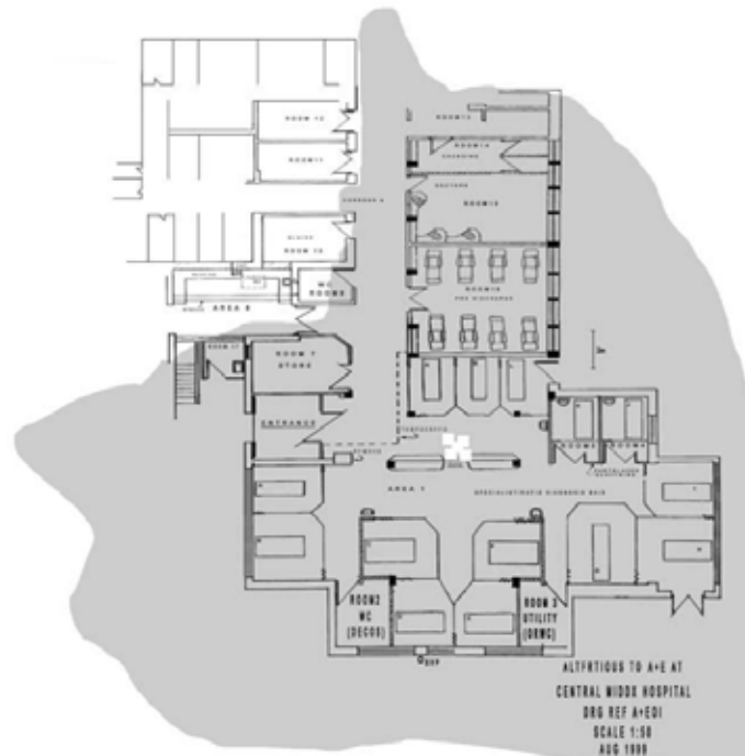
Coverage of a single AP (at 1Mbps) placed in the A&E majors room (marked white)
