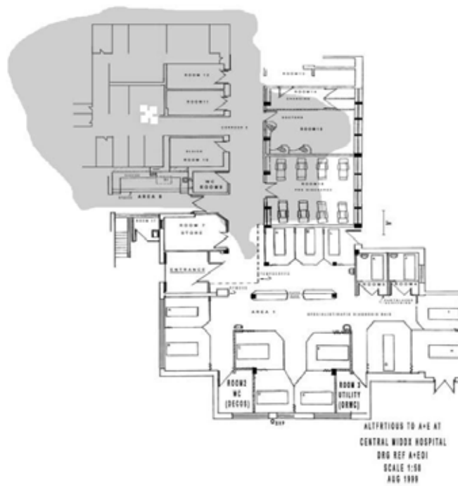
Coverage of a single AP (at 1Mbps) placed in the A&E minors room (marked white)
