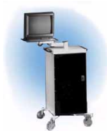
Fig. 4.1 A modern videoconferencing system including monitor, desktop computer (inside), camera and ISDN modem
