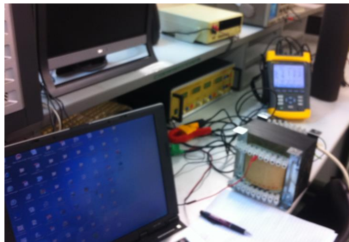
Photo 4.2: Practical testing through V_{ac} mains variations on PC - Laptop load.
