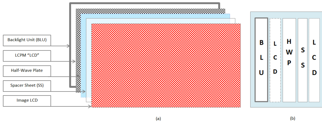
Figure A.12 – Block diagram of 2D/3D Switchable Content Adaptive H3D Display: (a) front view, (b) side view
