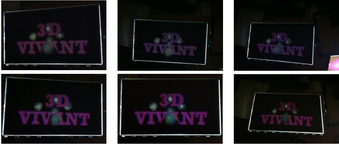
Figure A.30 – Playback result of full parallax holoscopic 3D display: Images captured from various angle
