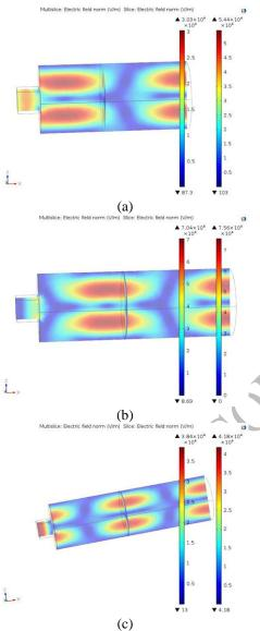
Fig. 8 Efield for various dimensions of the cavity (a) 333mm (b) 433mm and (c) 533mm
