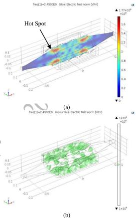
**Figure 4:** Electric field distribution (V/m) (a) ZX plane (b) 3D Iso-surface plot
