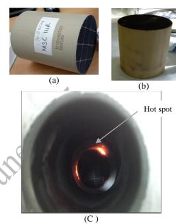
**Figure 2:** DPF at various stages (a) Clean DPF (b) Soot filled DPF and (C) DPF in microwave filed with glow.
