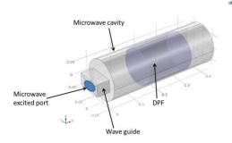
**Figure 5:** COMSOL geometry of the proposed microwave cavity
